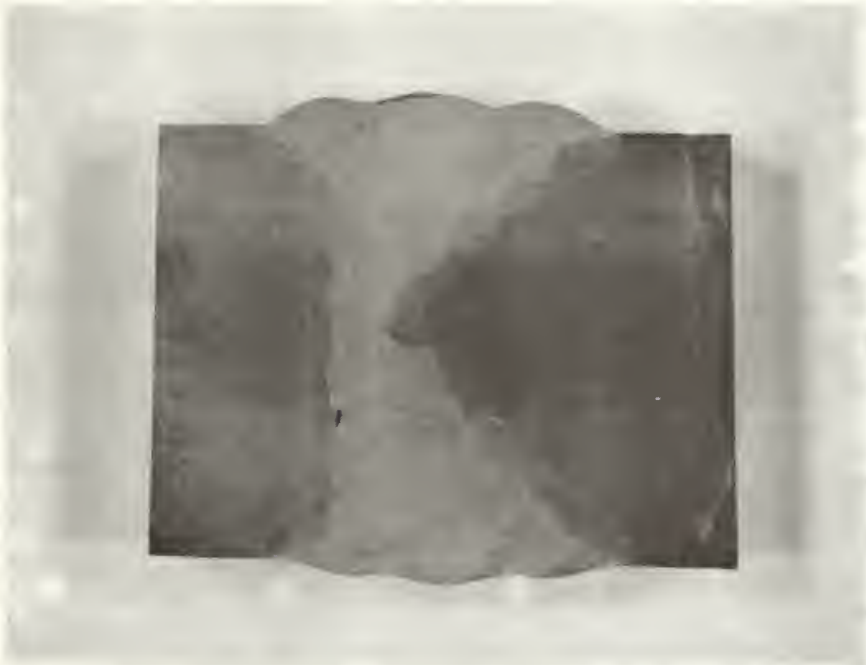
FIGURE 22 - Macroscopic Etched Surfaces of Gas Metal Arc (GMAW) and Submerged Arc (SAW) Welds.
