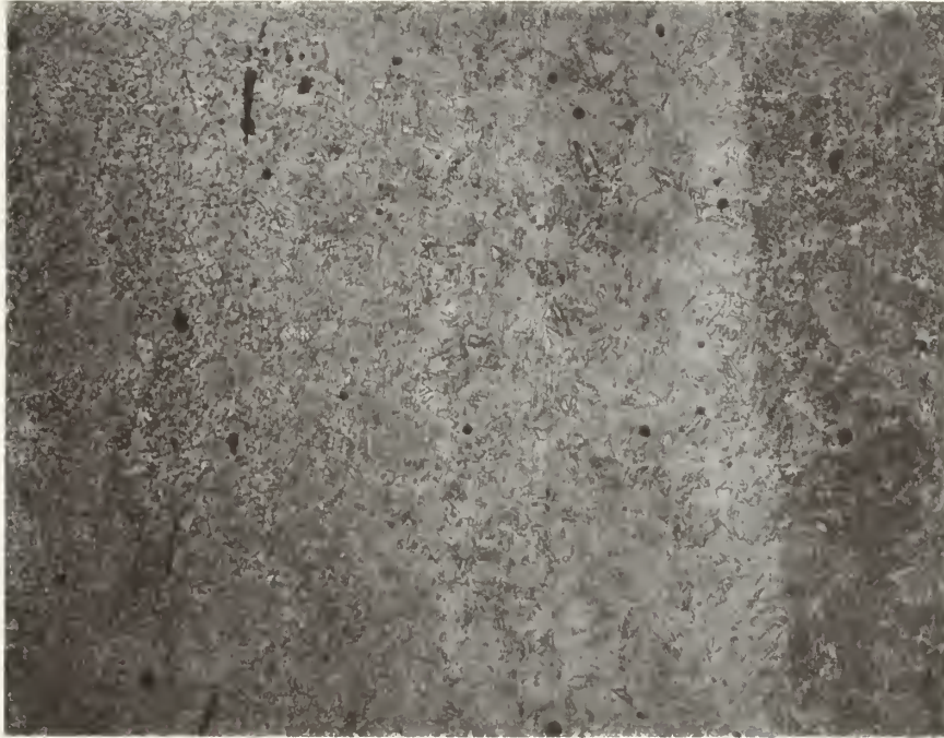
FIGURE 16 - Photomicrograph of Weld Region Showing Base Metal, Heat-Affected Zone and Weld Metal Grain Size Effects (100 X).
