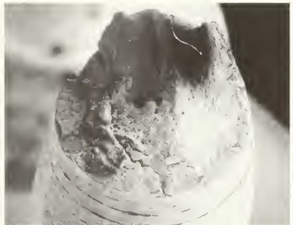
FIGURE 60 - Photomicrographs of Fracture Surfaces of Base Metal (top), GMA Weld Metal (middle left), GMA HAZ (middle right), SAW Weld Metal (bottom left) and SAW HAZ (bottom right) Showing Effect of Material (25 X). Strain Rate .0000667/sec, Applied Potential -1250 mv SCE.
