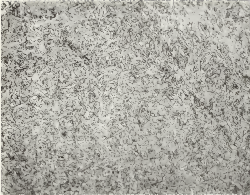
FIGURE 17 - Photomicrograph of Weld Metal Region (625 X).
