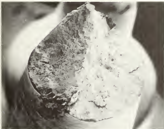
FIGURE 60 - Photomicrographs of Fracture Surfaces of Base Metal (top), GMA Weld Metal (middle left), GMA HAZ (middle right), SAW Weld Metal (bottom left) and SAW HAZ (bottom right) Showing Effect of Material (25 X). Strain Rate .0000667/sec, Applied Potential -1250 mv SCE.
