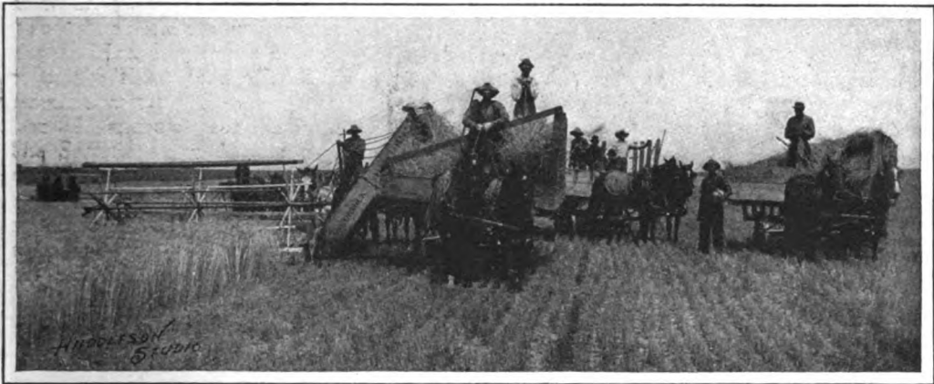
THE "HEADER" CUTS A VERY WIDE SWATH, LOADING WHEAT HEADS IN ACCOMPANYING WAGON, TO BE HAULED TO THRESHER, AND LEAVING THE STRAW IN THE FIELD
