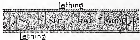
Section of Sound-Proof and Fire-Proof Partition
