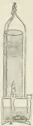
Fig. 1. Davy Lamp. solder; and the security depends upon the circumstance that no aperture exists in the apparatus larger than in the wire gauze.' The oil is supplied to the interior by the pipe projecting from the right side of the figure, and the wick is trimmed by a wire bent at the upper end, and passed through the bottom of the lamp, so that the gauze need not be removed for
