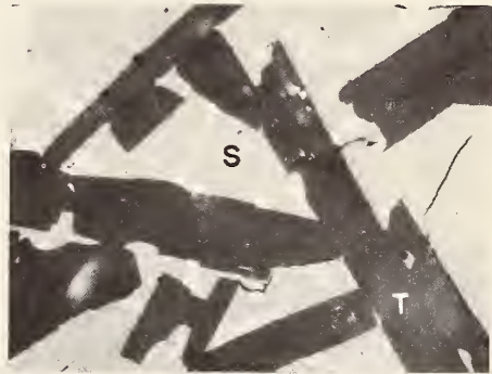
FIGURE 25. Euhedral growth. Example: tridymite ( \text{SiO}_2 ) in a silica-saturated iron oxide liquid (X169). In many situations the rate of growth is sensitive to crystal direction. T - tridymite; S - silicate glass.
