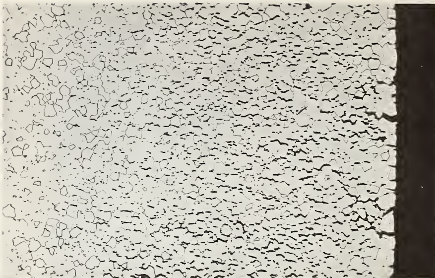
Figure 15. Generation of intergranular voids during torsional creep of high density alumina. (courtesy R. L. Coble).
