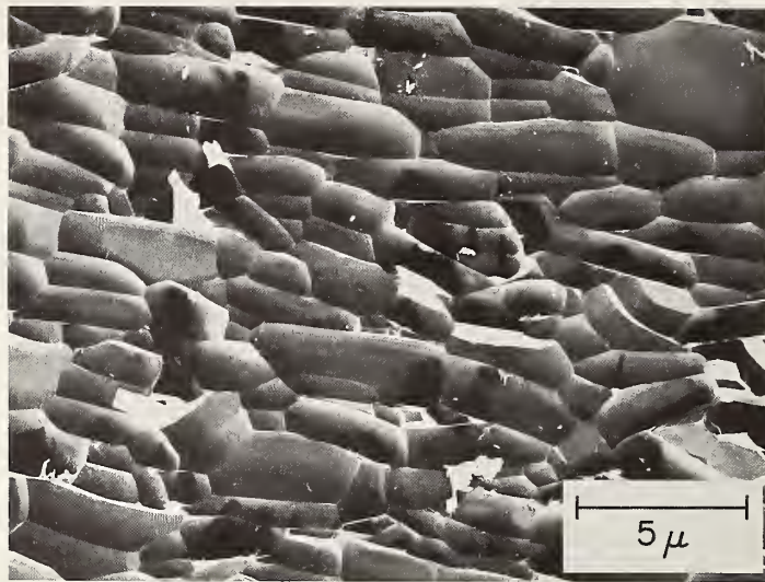
FIGURE 18. Photomicrograph of a crystal-oriented barium hexaferrite sample, thermally etched.
