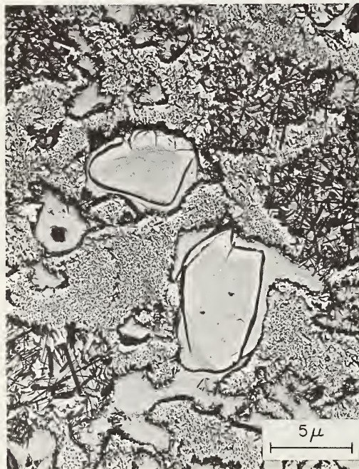
FIGURE 5. Two examples (a and b) of electron micrographs of electrical insulator porcelain (etched 10 sec, 0 °C, 40% HF, silica replica).
