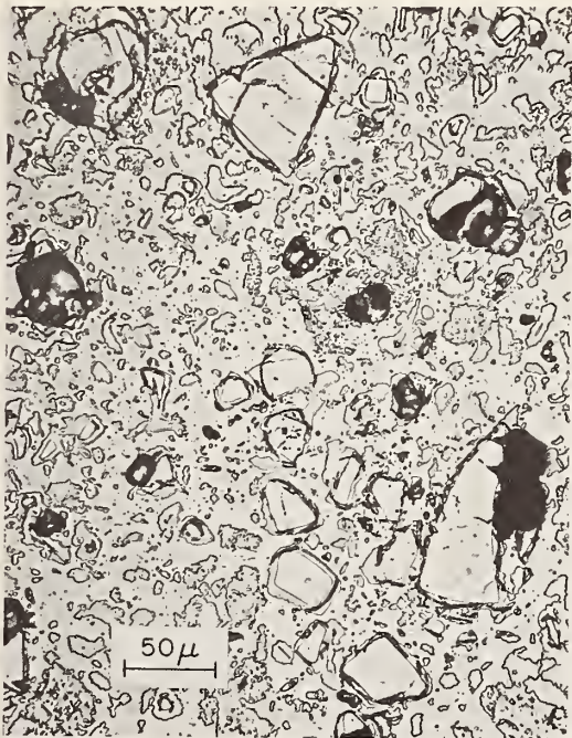
FIGURE 1. Electrical insulator porcelain with extensive quartz grain dissolution (etched 10 sec, 0 °C, 40% HF, collodion replica).
