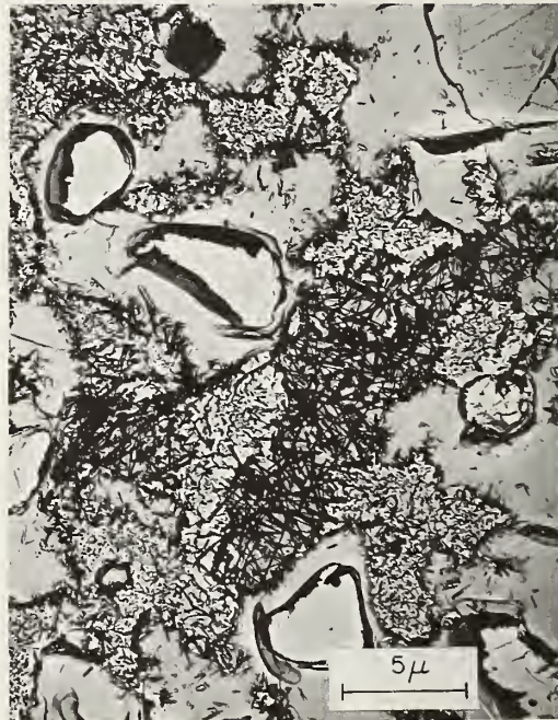
FIGURE 5. Two examples (a and b) of electron micrographs of electrical insulator porcelain (etched 10 sec, 0 °C, 40% HF, silica replica).
