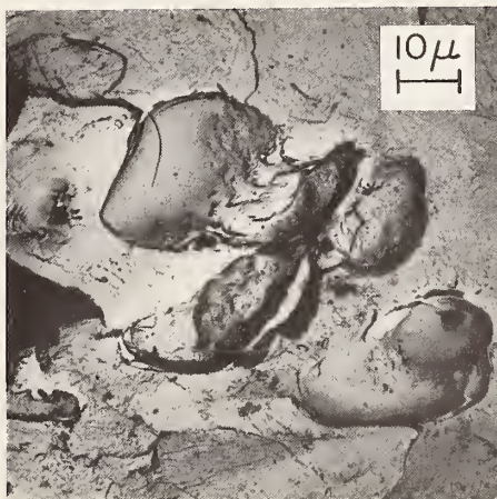
FIGURE 12. Stereoscopic views of closed pores in an unetched fracture surface (aluminium replica).
