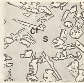
FIGURE 23. Grain shape (plates). Example: corundum ( \text{Al}_2\text{O}_3 ) in an alumina-saturated silicate glass (X281). The elongated shapes are cross-sections of the plate. Those plates which lie parallel to the surface are nearly equidimensional in the microsection. C - corundum; S - silicate glass.
