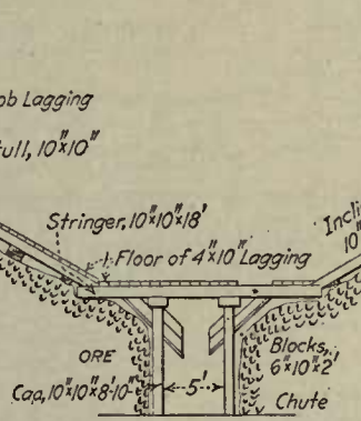
Fig.2 Regular Section Timbers
