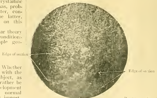
FIG. 1.—Chisel, from point. Longitudinal section. Magnified 50 diameters.
