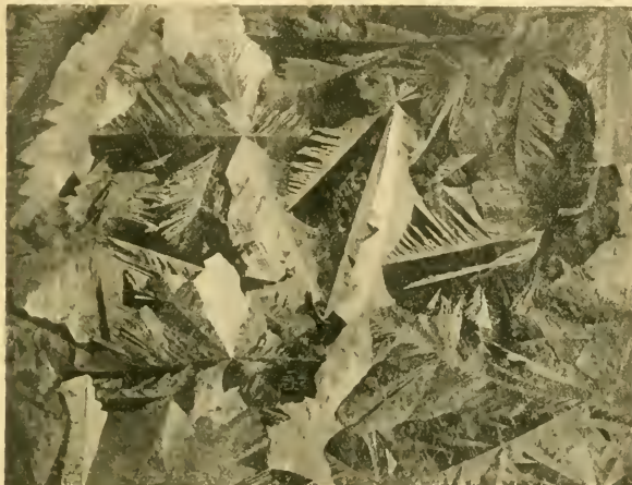
FIG. 1.—Surface of galvanized iron.
