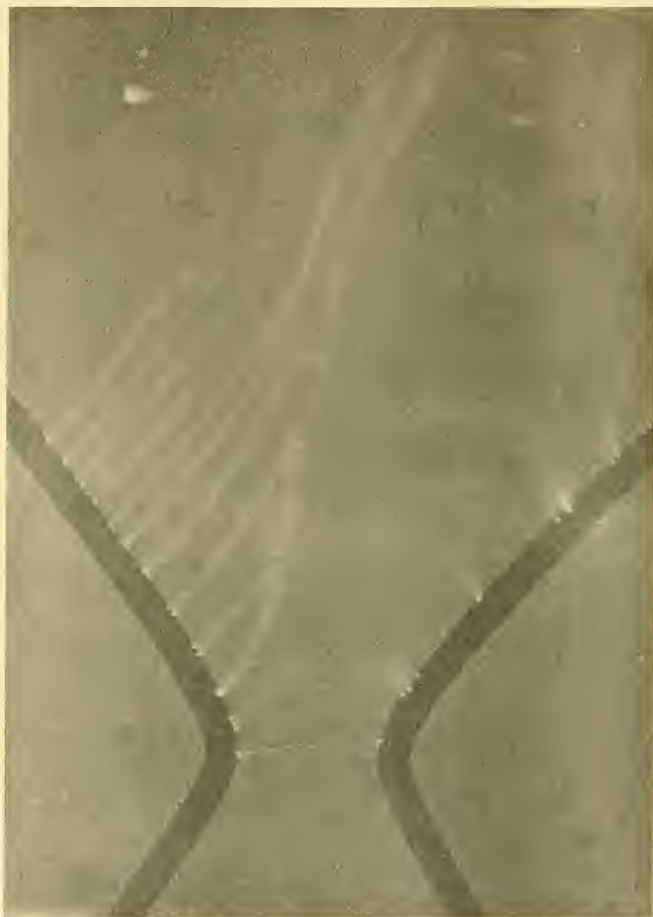
FIG. 4.—Arc flame between horn electrodes. From photograph by Mr. Lustgarten of Manchester.
