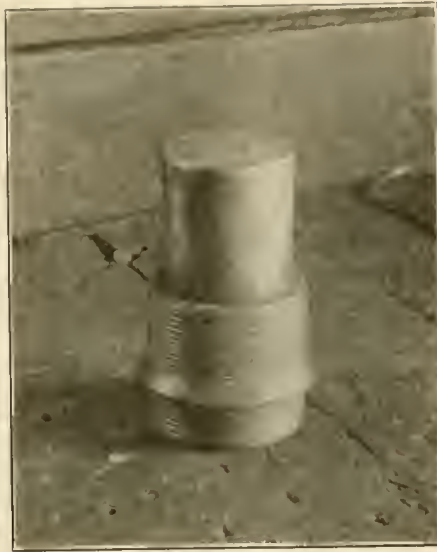
EXPANDER PLUG, READY TO BE DRIVEN INTO PLACE.
