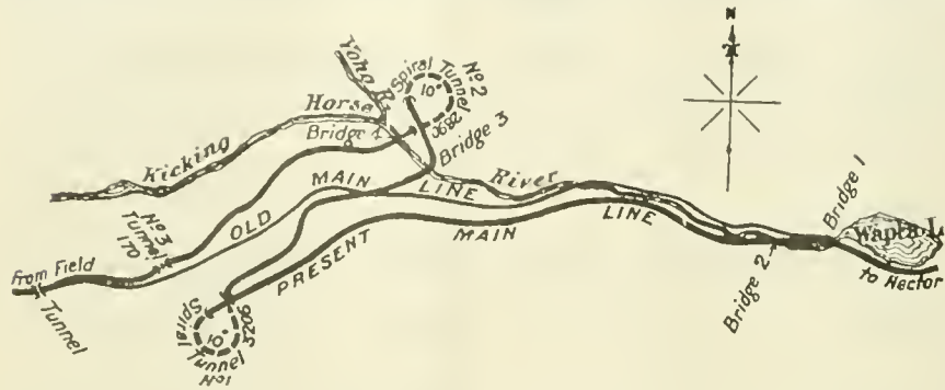
FIG. 1. GRADE REDUCTION WORK ON THE CANADIAN PACIFIC RAILWAY BETWEEN HECTOR AND FIELD, B. C.
