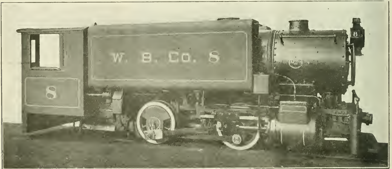
FOUR-COUPLED SWITCHER FOR THE WORTH BROTHERS COMPANY.
