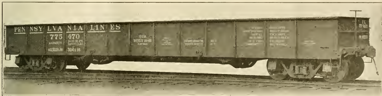
HEAVY FREIGHT GONDOLA CARS FOR THE PENNSYLVANIA RAILROAD. PRESSED STEEL CAR COMPANY, BUILDERS.
