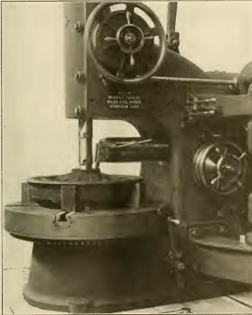
CAR WHEEL BORER, SHOWING HUB-FACING ATTACHMENT.
