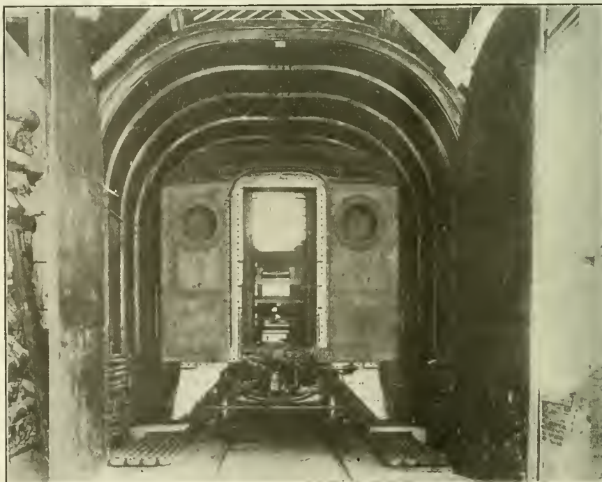
VIEW OF OVEN, OPENED, AND PAINTED CAR ABOUT TO BE REMOVED.
