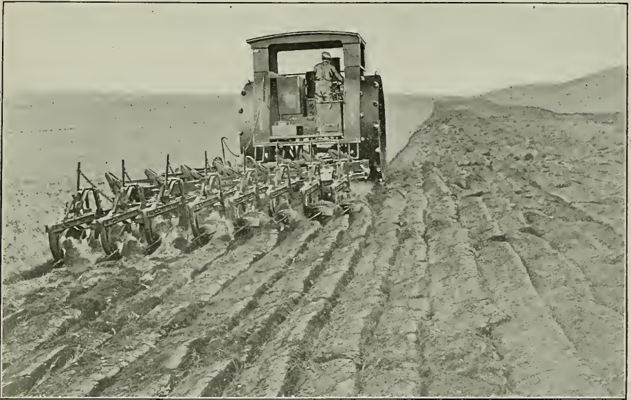
Avery Tractor—Breaking up the prairie—With the breaker bottoms the sod is turned over in long ribbons, as shown.
