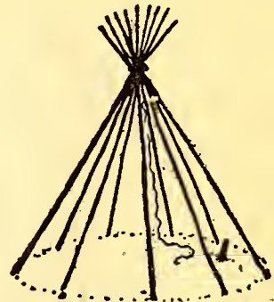
2 nd Set up & bind other six poles
