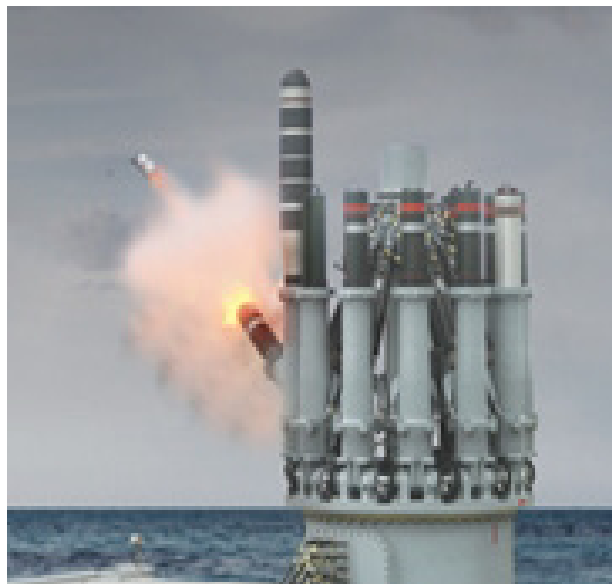
Figure 15. Centurion Launcher without Cover Installed. Source: Chemring Countermeasures (2013b).
