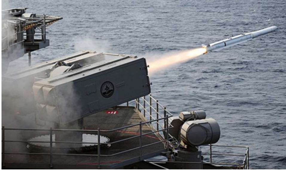
Figure 21. ESSM Launch from Mk 29 Launching System. Source: Rogoway (2017).
