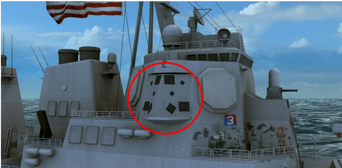
Figure 11. SEWIP Block 3 Antennas (Circled in Red). Adapted from Northrop Grumman (2019).
