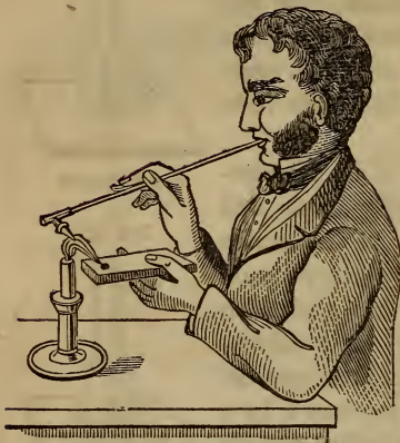
Using the Blowpipe.
