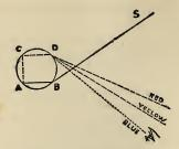
Here the ray SB (of the secondary rainbow) strikes the drop at B, is refracted to A,—is then reflected to C,—is again reflected to D, when it is again refracted or bent, till it reaches the eye of the spectator.
