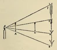
Here the arrow A held close to the candle, will cast the shadow PB on a wall; while the same arrow held at C would cast only the little shadow DE.  $\times a$
