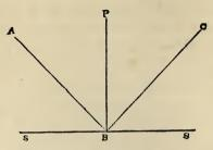
Let SS be any surface, PB a perpendicular to it—If a marble were thrown from A to B, and bounded back to C; then ABP would be called the angle of *incidence*, and CBP the angle of *reflection*.
