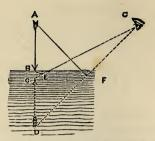
there the arrow head A strikes the water at F, and is reflected as if from D; and the barb B strikes the water at E, and is reflected as if from C.
