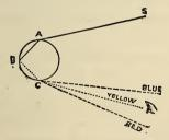
Here the ray SA (of the primary rainbow) strikes the drop at A,is refracted or bent to B,- is then reflected to C, where it is refracted again, and reaches the cyc of the spectator. (See p. 414.) N B 3
