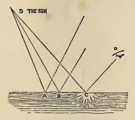
Here, of the rays SA, SB, and SC, only the ray SC meets the eye of the spectator D. If a line were dropped perpendicularly over C, the angles formed between that line and SC, and DC, would be equal.
