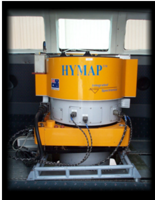
Figure 10. HyMap sensor mounted in Cessna style aircraft. From http://www.intspec.com on October 13, 2006.
