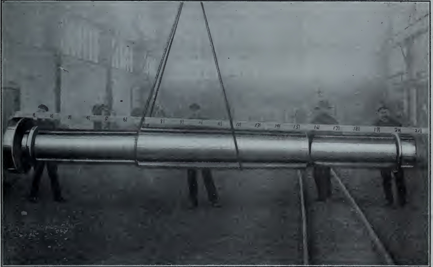
FINISHED COUPLING SHAFT, 18 IN. DIAMETER BY 21 FT. LONG.
