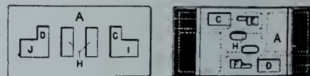
FIG. 11. UPPER—AUXILIARY VALVE. LOWER LEFT—MAIN VALVE FACE. LOWER RIGHT—FACE ON BACK OF MAIN VALVE FOR AUXILIARY VALVE.
