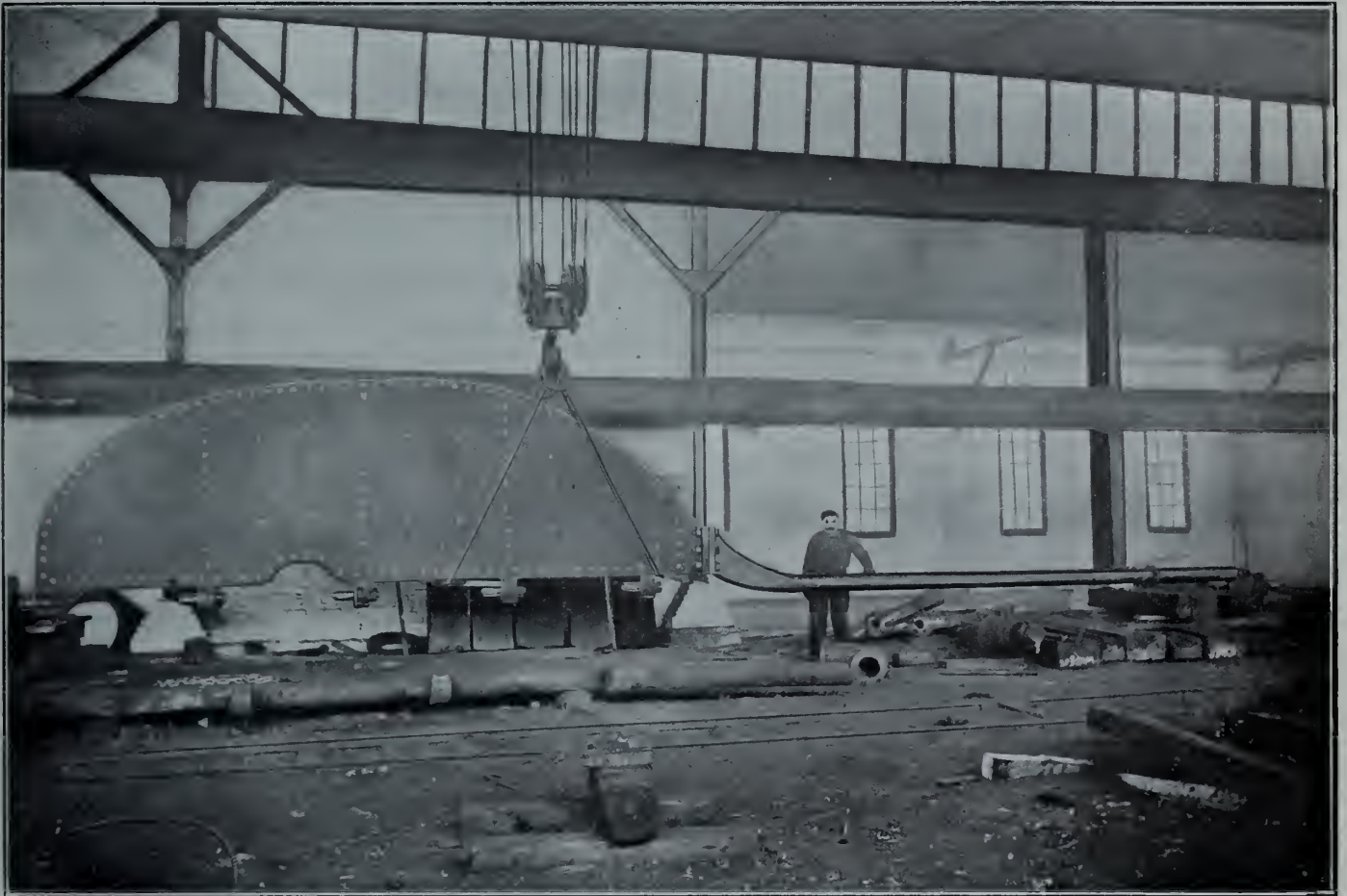
RUDDER FOR SS. "LUX." WEIGHT 9 TONS, LENGTH 42 FEET.
