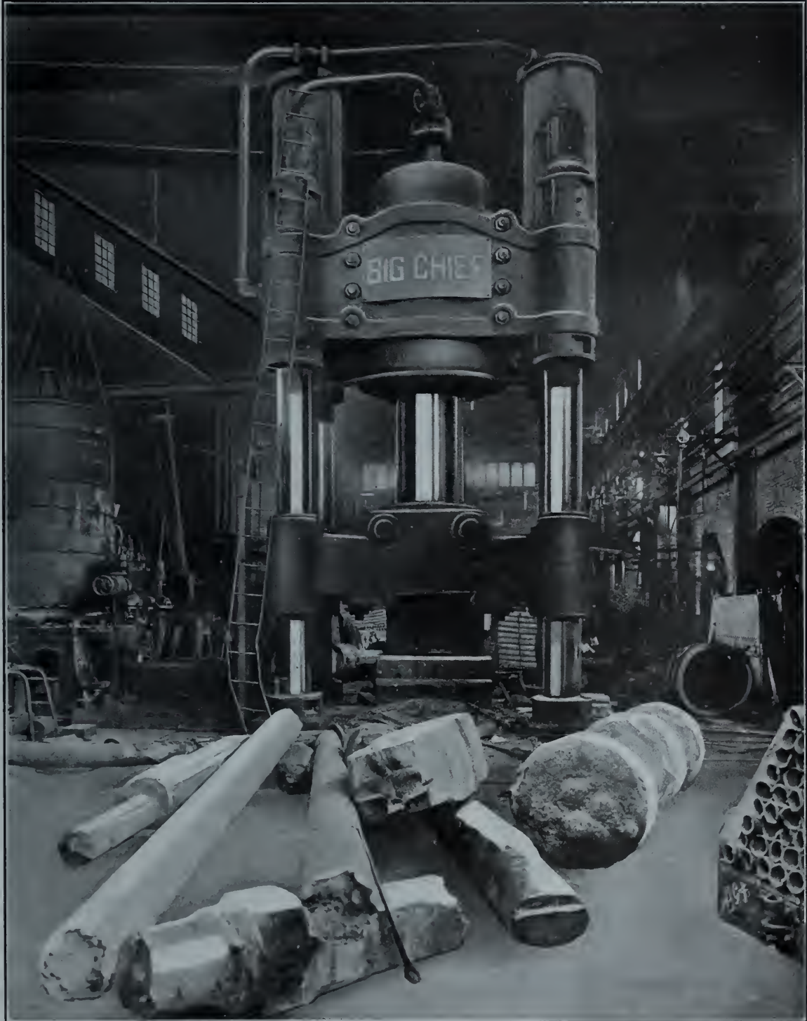
4,000 TON STEAM HYDRAULIC FORGING PRESS FOR MARINE AND OTHER HEAVY FORGINGS.
