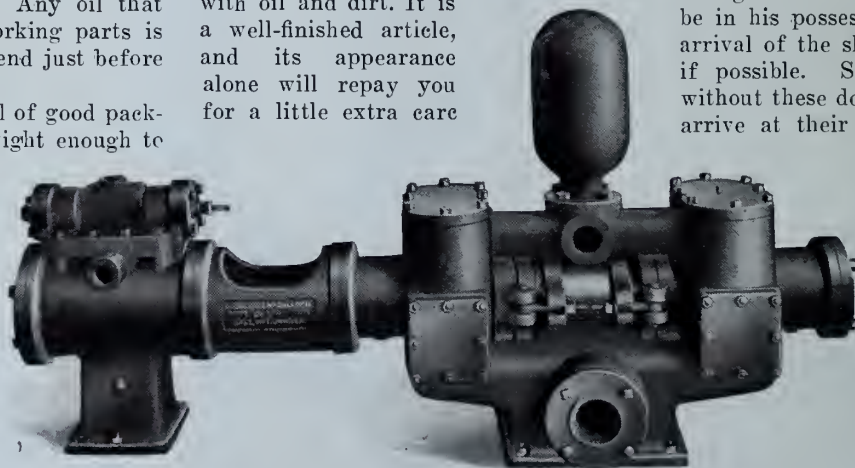
"GOLDIE & McCULLOCH" OUTSIDE PACKED, PLUNGER TYPE, BOILER FEED PUMP.
