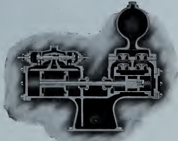
FIG. 13—TYPE B TO D "MARSH" PUMP IN SIZES 2½ X 1½ X 2 IN. TO 5 X 3 X 3½ IN.
