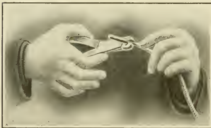
"Crimp" or fasten caps to fuse with a regular crimping tool. This tool does the job far better than it can be done in any other way.
