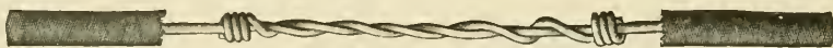
Very best wire connection, ready for soldering if need be. (Excellent for leading wire.)
