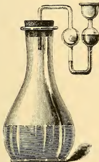
FIG. 135.—Flask for the Approximate Estimation of Sugar by Fermentation (1).
