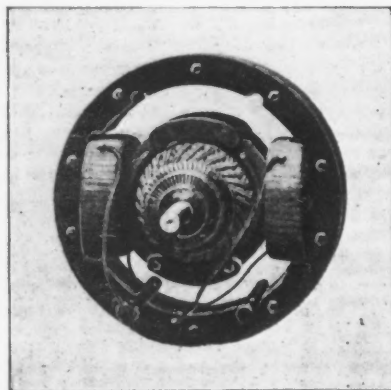
Fig. 2.—View Showing Removable Field Ring Pole Pieces and Armature.
