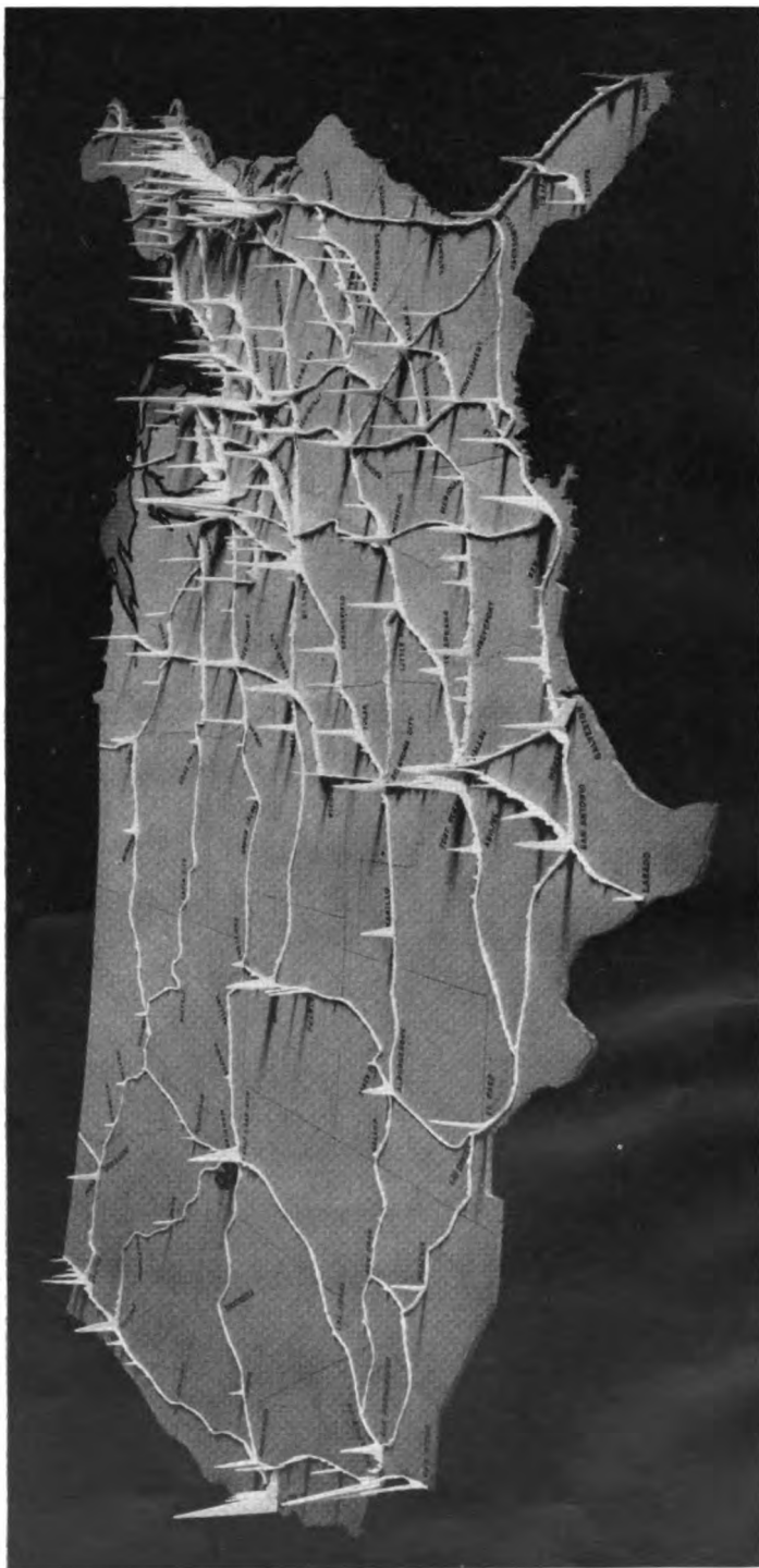
FIGURE 22.—Relief traffic map of the recommended interregional system. The height of the traffic bands indicates approximately the average density of traffic to be expected at all points on the system. The mounting spires at the principal cities picture the great increases of traffic to be expected on sections of the routes traversing the cities.
