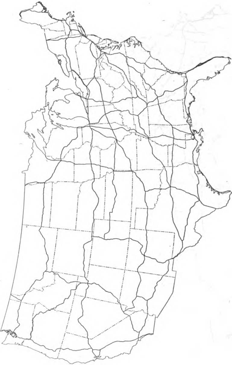
FIGURE 2.—The 26,700-mile system tentatively proposed as an interregional highway system by the Public Roads Administration in the report, Toll Roads and Free Roads .
