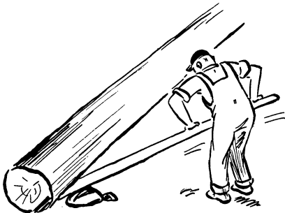
Figure 59.—Prying the butt back sometimes frees a lodged tree.
