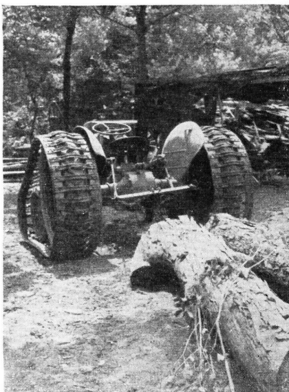
Figure 2.—Accessory crawler tracks on a wheel tractor give much better traction in mud or snow.
