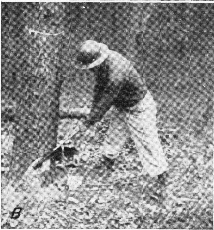
Figure 10.—Stance for chopping: A , Top of ax stroke. Notice the position of the hands. B , End of ax stroke. The upper hand slides down the handle during the swing.
