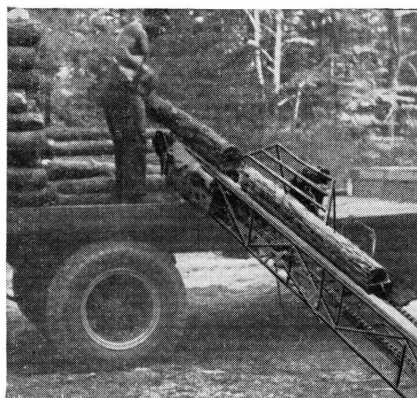
Figure 44.—An inexpensive pulpwood conveyor-loader makes this job easier.
