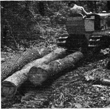
Figure 4. —The small crawler tractors can be used as dual-purpose machines, for farm work as well as logging.
