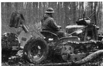
Figure 41.—A small logging sulky suitable for use with a small tractor.
