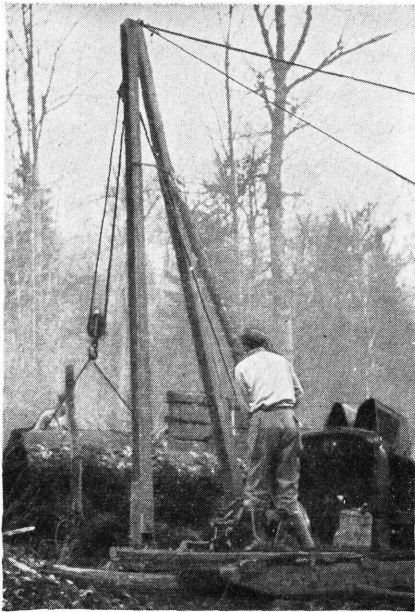
Figure 83.—An A-frame jammer can be homemade.
