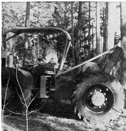
Figure 3. —One of the new 4-wheel-drive tractors, equipped with a winch and integral arch for logging. With the winch logs can be dragged out of places where a tractor cannot be taken.
