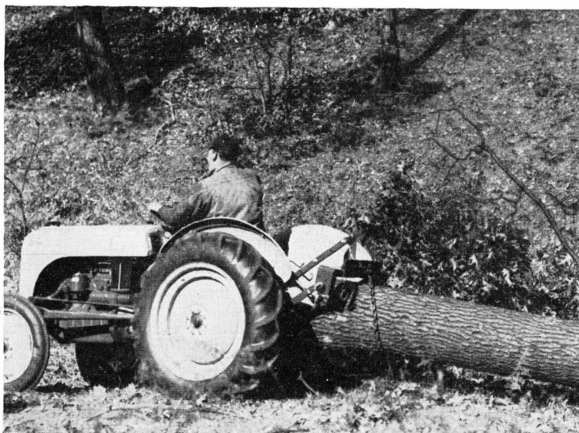
Figure 1.—An ordinary farm tractor can be used on many logging jobs. Note how the hydraulic-lift drawbar is used in skidding the log. (Slope in the background of this area is hazardous for the use of a wheel tractor.)
