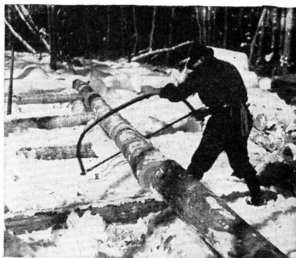
Figure 61.—Bucking at a landing with a bow saw. Notice the skids, which keep the tree stem off the ground.
