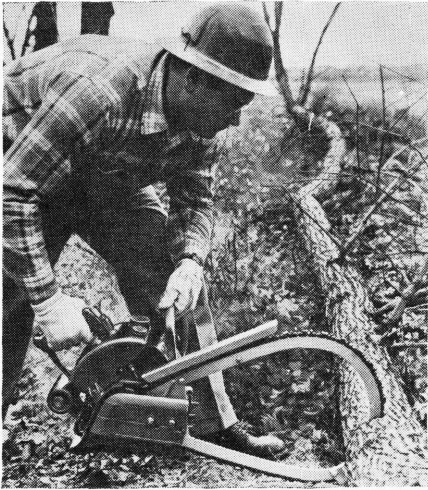
Figure 32. —The bow type of chain-saw bar is widely used for cutting small timber. In bucking especially, there is little chance of pinching and little need of wedging with this type of bar.
