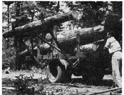
Figure 85.—The "timber tosser" flips logs up onto the truck.
