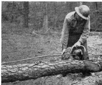
Figure 62.—With a measuring rod attached to the chain saw, measure while cutting.
