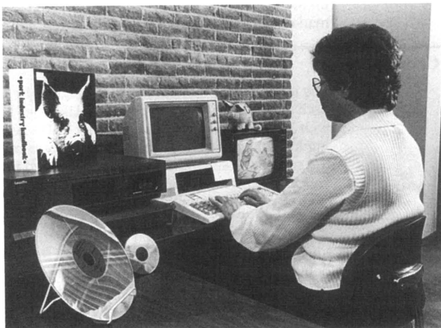
The National Agricultural Library, in cooperation with other institutions, is evaluating the use of 12-inch laser discs as a means for storing, retrieving and disseminating information from agricultural publications. A 12-inch disc and a smaller one, which resemble phonograph records, are at the left. (William E. Carnaban)
