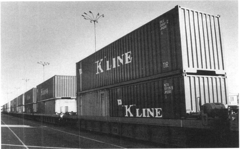
Double-stacked container rail cars mean that more containers can be placed on each railroad freight car. Thus, more containers can be carried on each train. Such container movements expanded from 30,000 in 1984 to more than 400,000 in 1987. (June Davidek)
