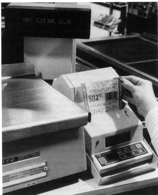
Some supermarkets have coupon-producing machines at the cash register. As the shopper's order is processed, the coupon dispenser determines if there are related or competing items in the system and prints out corresponding coupons that can be redeemed on the next shopping trip. (Giant Food, Inc.)
