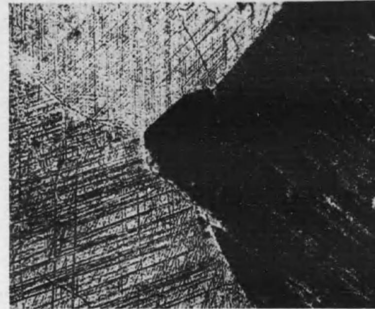
Photo. 26 The same portion as Photo. 25 after tempering for 1 hr. at 240^{\circ}\text{C} . Etched with Keller's reagent. \times 120
