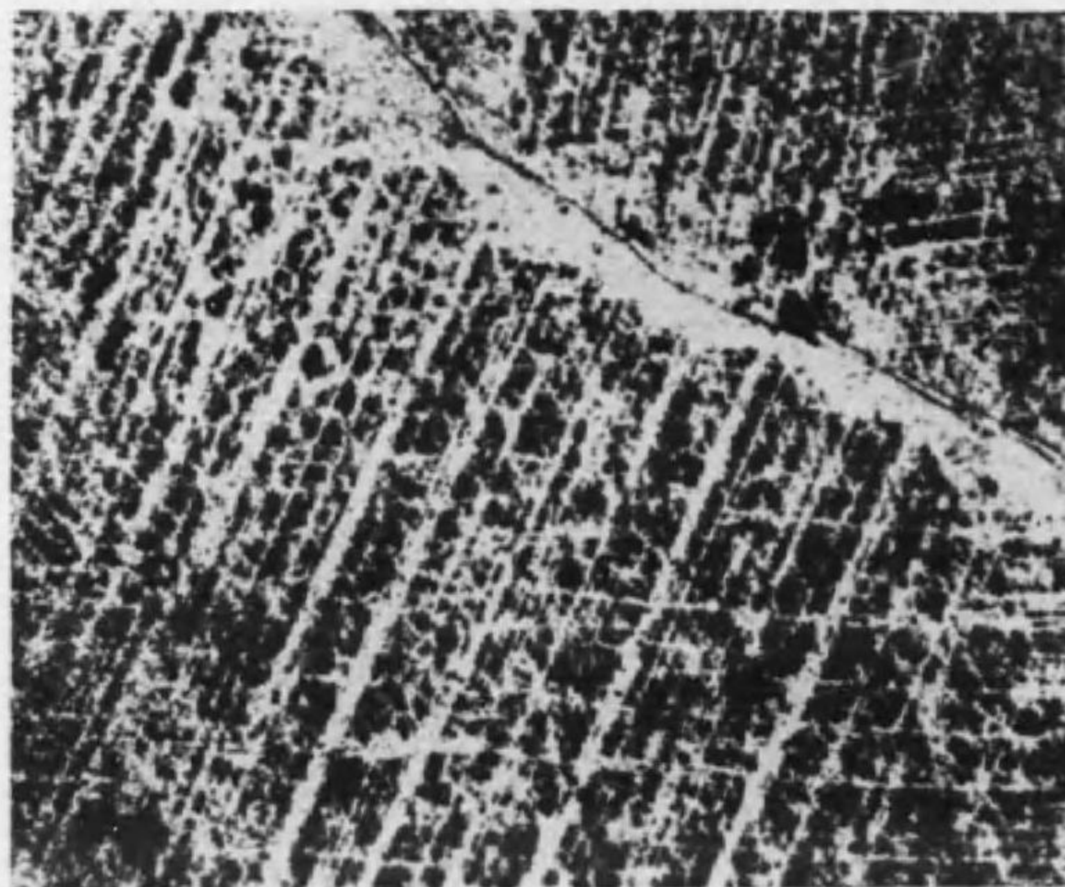
Photo. 29 4% Cu: quenched in iced water. Deeply etched with 1.5 normal HCl solution for 4 hrs. \times 120
