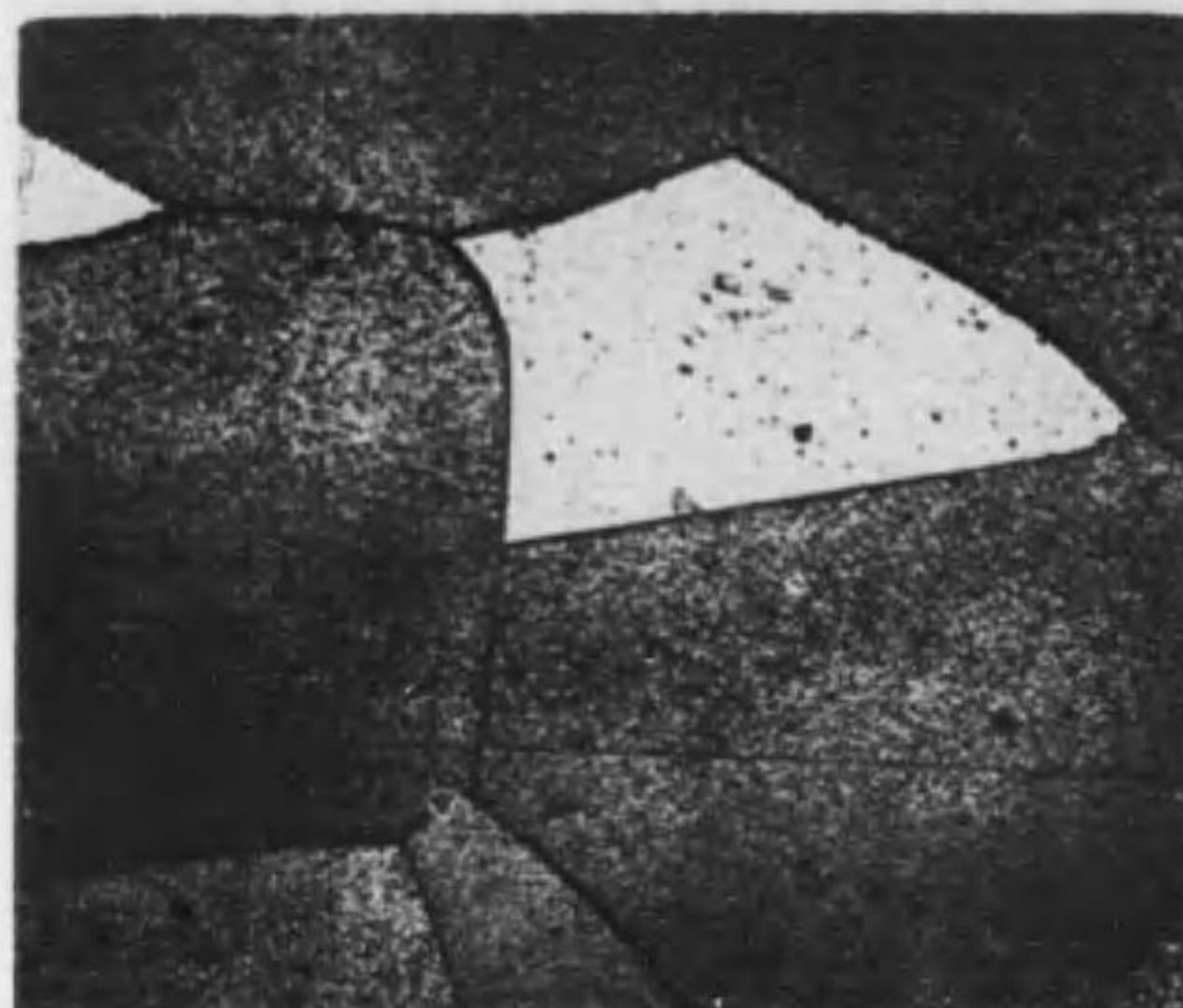
Photo. 21 1% Cu: tempered for 1 hr. at 250°C. after quenching in iced water. Etched with Keller's reagent. ×100
