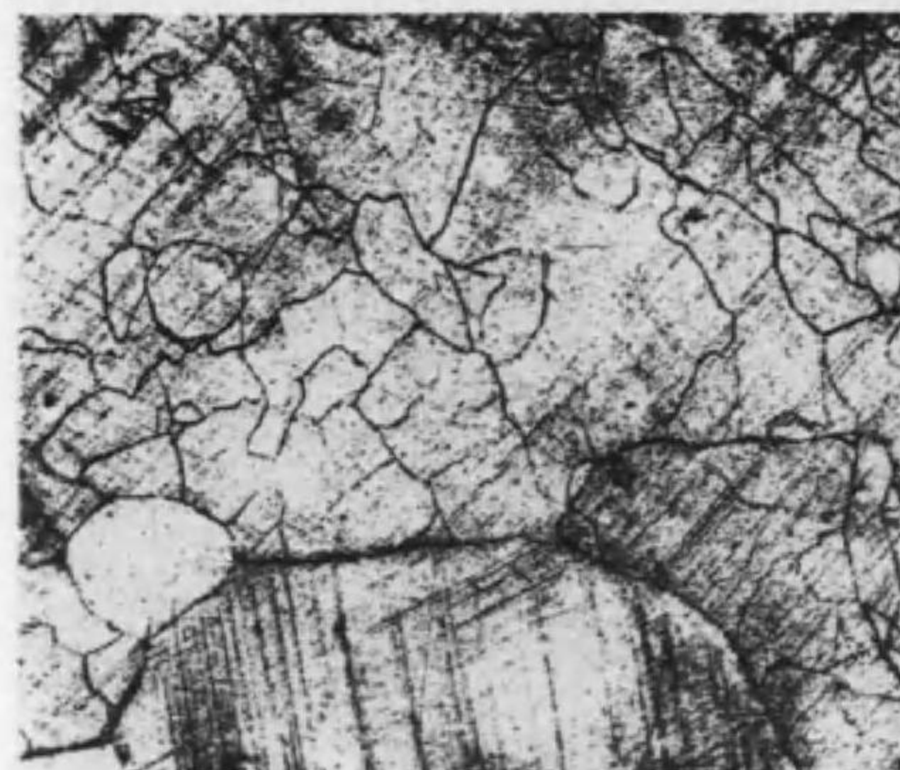
Photo. 23 1.5% Cu: tempered for 1 hr. at 250°C. after quenching in iced water. Etched with Keller's reagent. ×100
