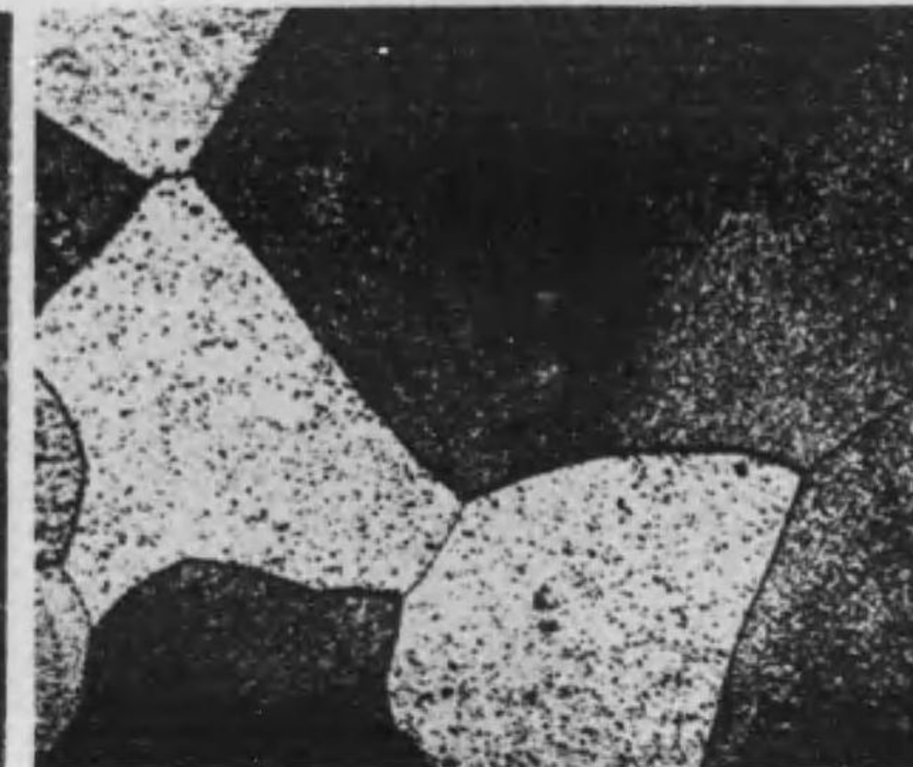
Photo. 22 1% Cu: tempered for 1 hr. at 300°C. after quenching in iced water. Etched with Keller's reagent. ×100
