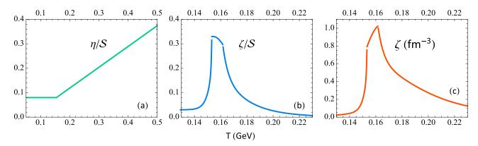
FIG. 2. The temperature dependence of (a) the specific shear viscosity  $\eta/S$ , (b) the specific bulk viscosity  $\zeta/S$ , and (c) the bulk viscosity  $\zeta$  itself in units of fm<sup>-3</sup>, given by the parametrizations (78) and (79) [6]. We note that the peak of  $\zeta/S$  in panel (b) occurs at the temperature  $T = 0.995T_c \approx T_c$  whereas the bulk viscosity  $\zeta = (\zeta/S) \times S$  in panel (c) peaks at the higher temperature  $T = 1.05T_c$ .
