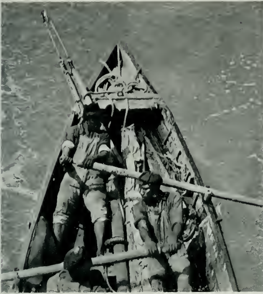
A few strokes put the little craft safely away from the ship. This photograph shows the mast and sail, two of the keen toggle irons resting on the gunwale, and the manila whale line which passes out through a notch in the bow. The men follow directions signaled to them by the captain
