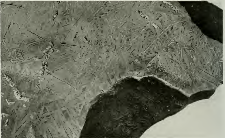
The iron meteorite has a very thin black crust, of metallic luster. The texture within remains unaltered by the fiery journey through the sky. On some iron meteorites peculiar crosslines, "Widmanstätten lines," may be etched with a weak solution of nitric acid
