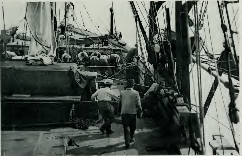
A chain passed through a starboard hawse pipe is fastened around the whale's "small," and when drawn in snugly, the victim lies with his flukes near the bow and his head stretching along past the waist. The operations of bringing a whale alongside and of making it fast are called sweeping and fluking. The boat hanging on the forward davits is the writer's dory, not part of the regular whaling equipment of the brig
