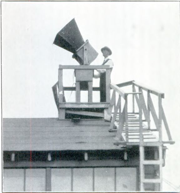
SKY BRIGHTNESS METER MOUNTED ON PLATFORM ON THE ROOF OF THE BUILDING.
