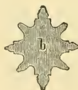
Profile of Piers in the Flamboyant Style. a. In the Church of St. Maclou at Rouen. b. In the Cathedral at Orleans.
