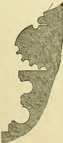
Profile of the base of a Column in the Temple of Minerva Polias at Priene.
