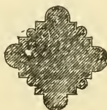
Plans of richer forms of Piers with Half-Columns. Moulded Piers.
