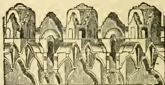
Section of part of the Roof of the Capella Palatina at Palermo.
