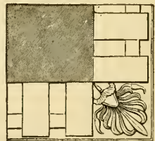
View of Corner-Dentels from beneath.
