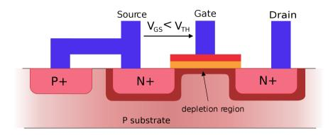
The 'metal' in the name MOSFET is now often a misnomer because the previously metal gate material is now often a layer of polysilicon (polycrystalline silicon).
