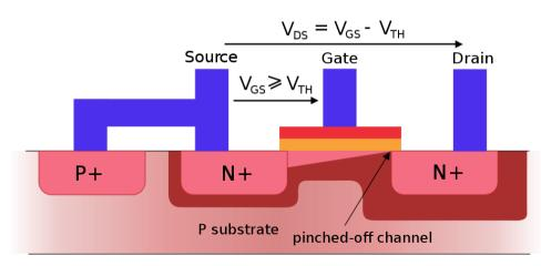
Saturation mode at point of pinch-off
