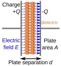
Charge separation in a parallel-plate capacitor causes an internal electric field. A dielectric (orange) reduces the field and increases the capacitance.
