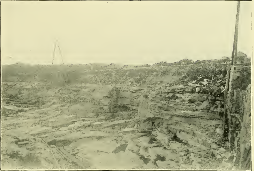
FIGURE 1.—EASTERN QUARRY OF THE SMITH GRANITE COMPANY AT WESTERLY, RHODE ISLAND The view shows the onion-like joints
