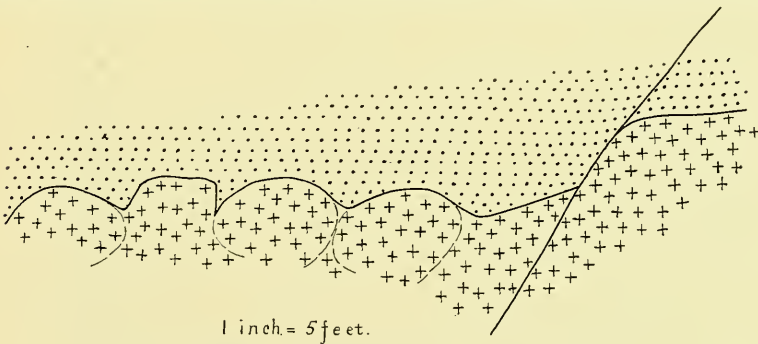
FIGURE 9.—Irregular Contact broken by a Fault.
