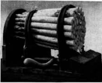
Figure 6.—One type of asparagus-bunching device. Note that the spears have been cut to a uniform length.
