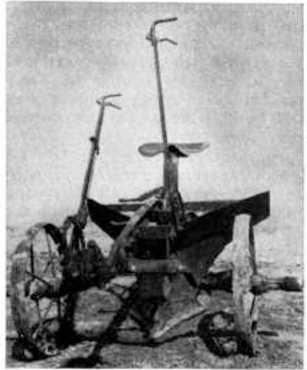
Figure 1.—This implement is one type used to open furrows for setting asparagus crowns. The blade can be adjusted to make furrows of the proper depth.
