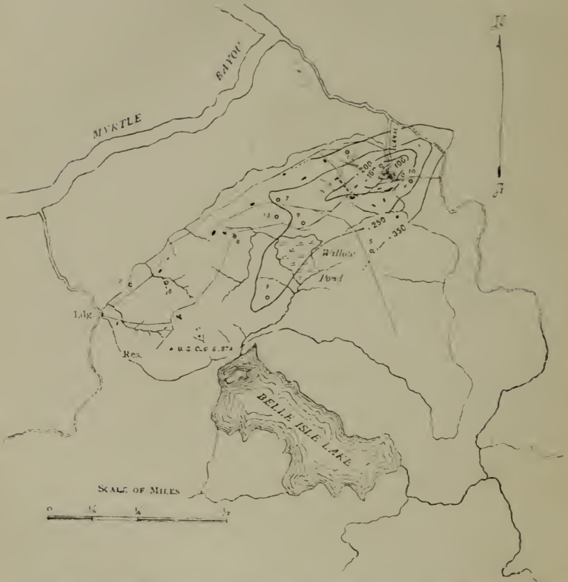
Contour Map of the Salt Deposit on Belle Isle. Elevation given in feet below Gulf Level
