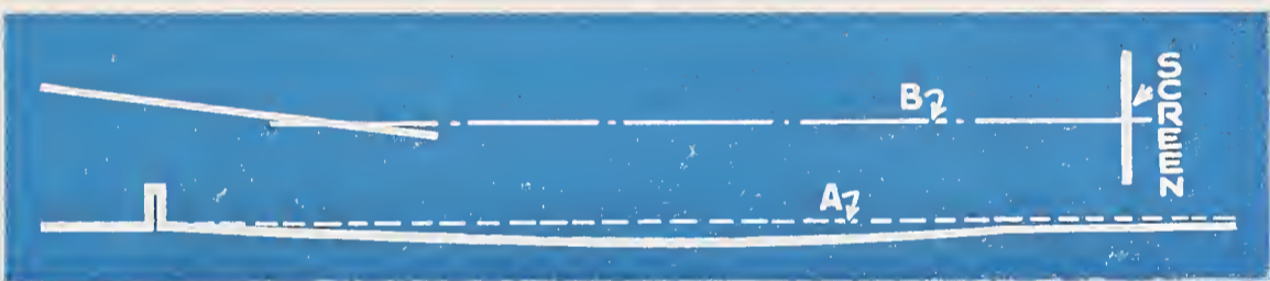
Below, the "dual incline" floor now used by the author, with a direction and pitch as conditions indicate
