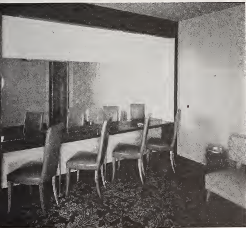
The women's cosmetic room is finished in plaster on three walls, with the fourth wall constructed of translucent glass block. The color scheme is peach with blue neon lighting. The cosmetic shelf is opaque architectural glass.
