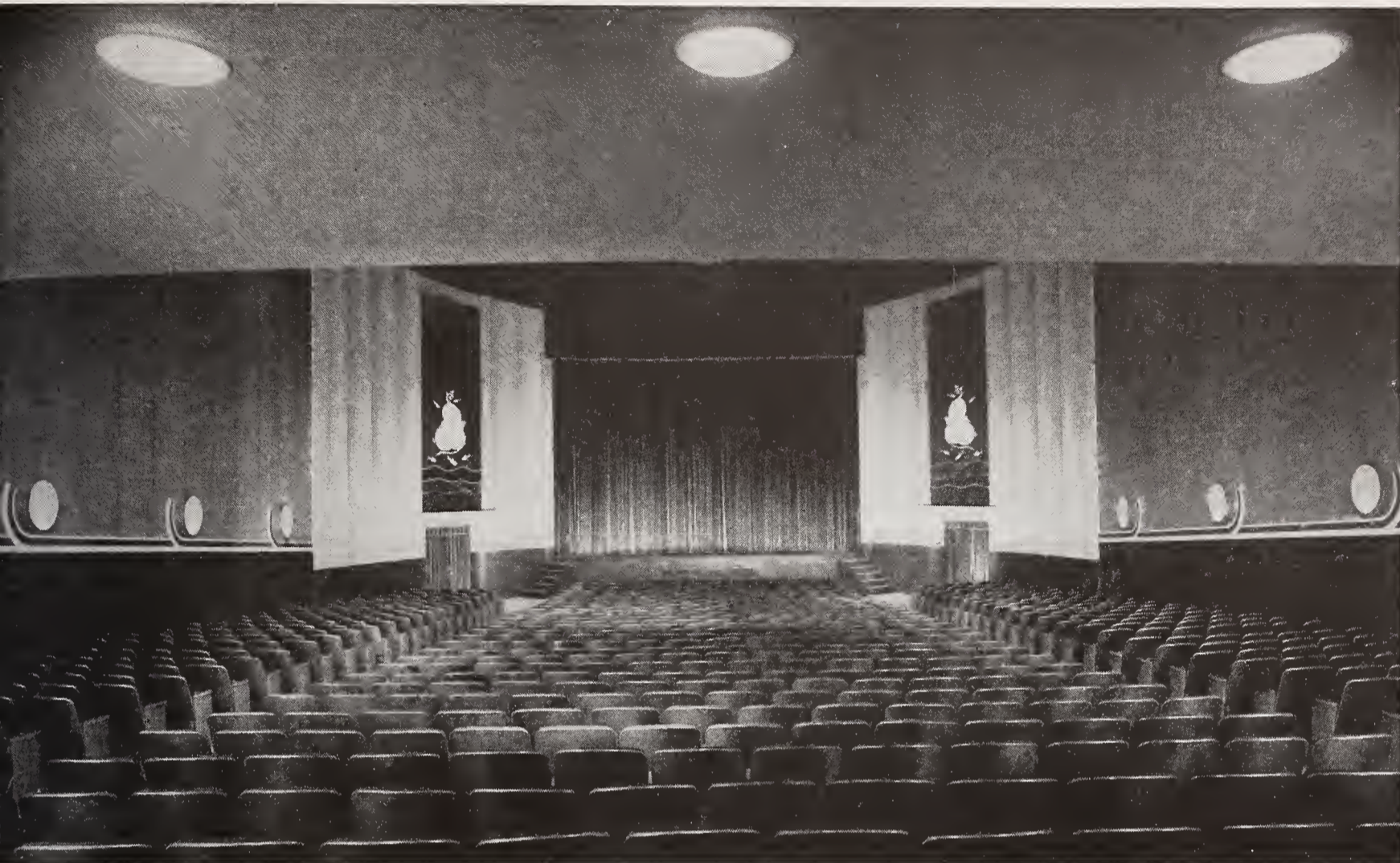
The auditorium of the Tipton theatre has sidewalls of fibreglas fabric, in wine color above a plum-colored wainscot. Pattern is supplied largely by the ceiling, with its numerous circular light troughs, some of them suspending Agitair air diffusers.
