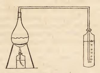
But it is not always necessary to prepare a watery solution of Sulphuretted Hydrogen, a stream of the gas, introduced into the suspected liquor by means of the above apparatus, will act with equal delicacy, and possesses as Dr. Christison has observed, the advantage of not diluting it. Before applying this test, it is necessary to add an acid, if any alkali should exist along with the Arsenic, otherwise no precipitate will take place.
