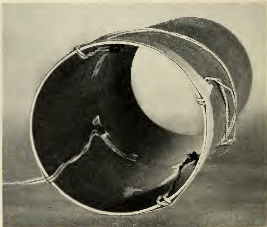
Fig. 1 — Thin-walled tube with SR-4 strain gages.
