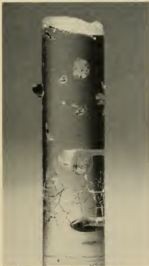
Fig. 9 — Section of Lucite rod showing penetration by pholads. One of the mollusks can be seen protruding from the left-hand side of the rod. Original magnification 2X.
