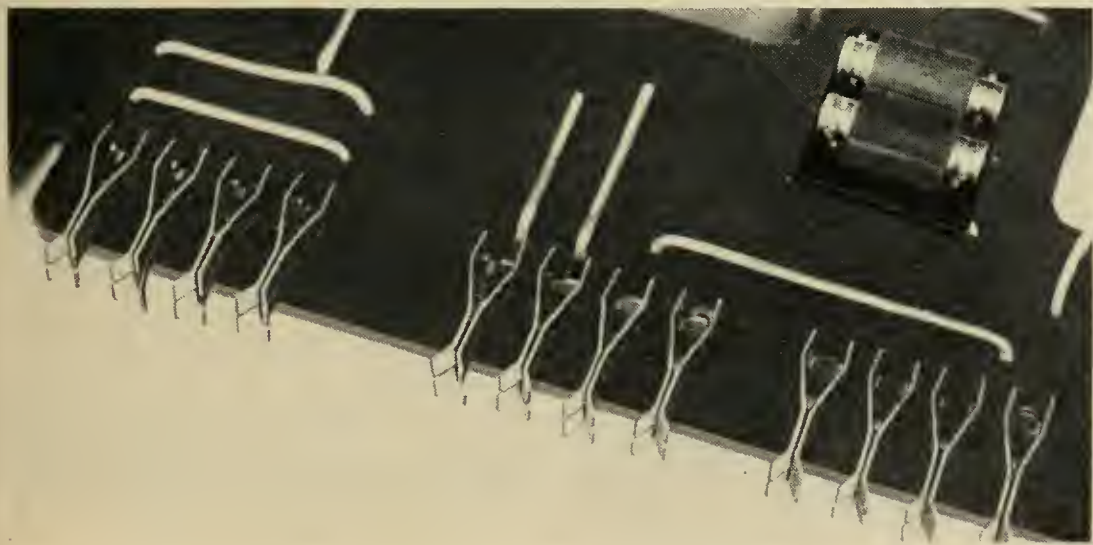
Fig. 16. — Closeup of terminal connectors.
