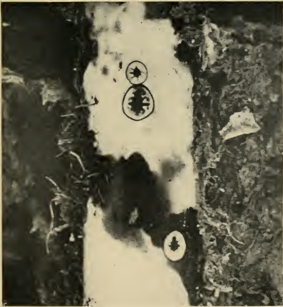
Fig. 13 — Sulfiding of Poly(Vinyl Chloride) plastic test rod beneath barnacles. The black, circular border and center area represent sulfiding at points of exceptionally close contact. Original magnification 2X. Photo by J. B. DeCoste.
