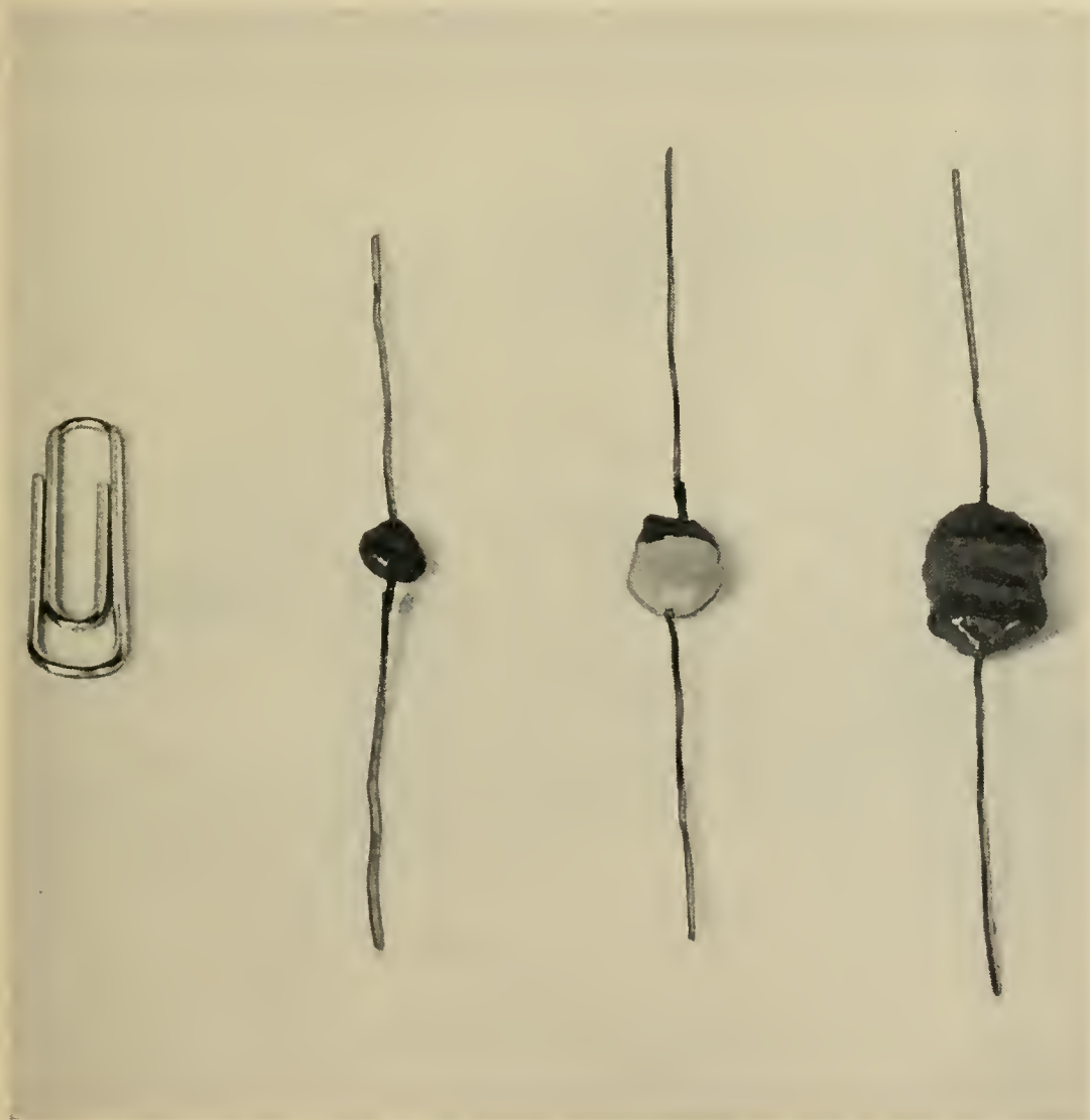
Fig. 12 — Prototype solid tantalum capacitors for P1 carrier.
