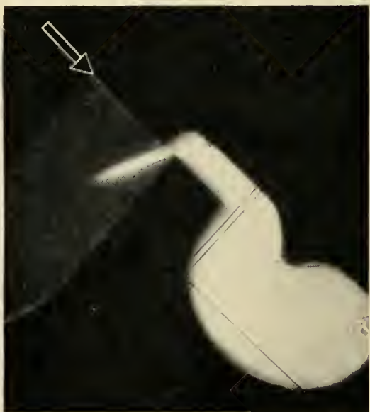
Fig. 17 — Flow through port with decreased Bernoulli effect and increased flow.
