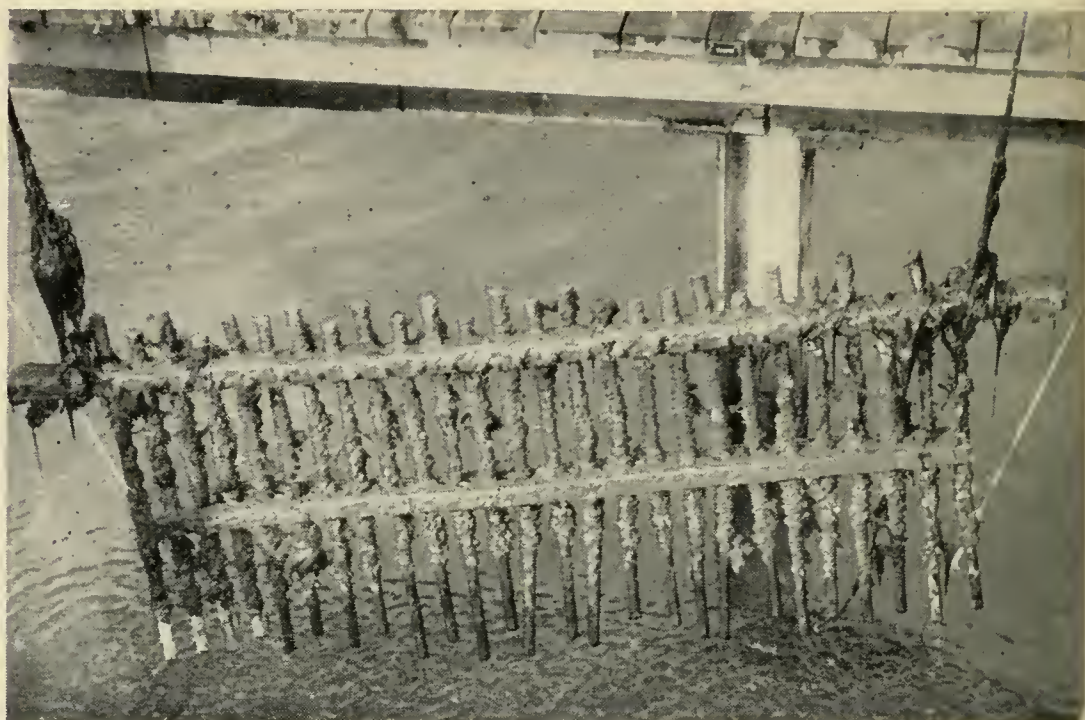
Fig. 12 — Test rack being lifted from water at Wrightsville Beach. Heavy accumulation of fouling on test rods in water-exposed area stops at point where rods entered the sediment.
