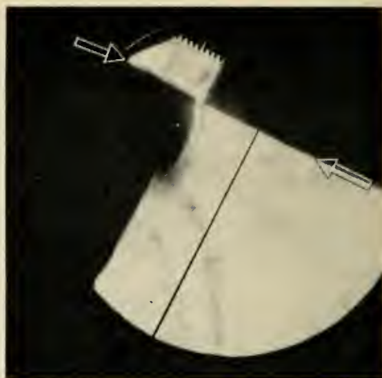
Fig. 15 — Oil flow through simple port.
