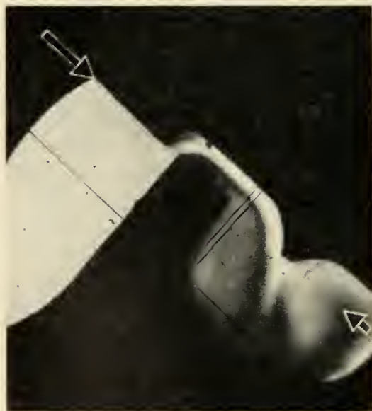
Fig. 17 — Flow through port with decreased Bernoulli effect and increased flow.
