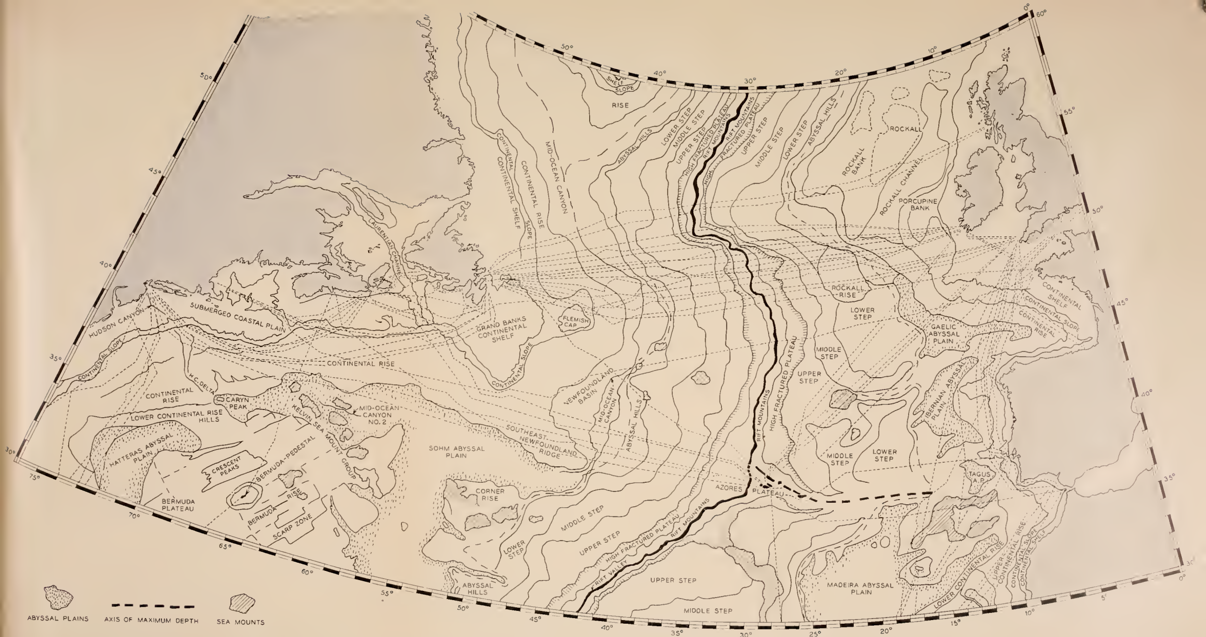
Fig. 6 — Great-circle chart showing physiographic provinces and existing submarine cable routes (dotted lines). (On this chart any straight line represents a great circle.)
