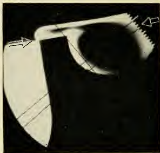
Fig. 16 — Flow through port with decreased Bernoulli effect.
