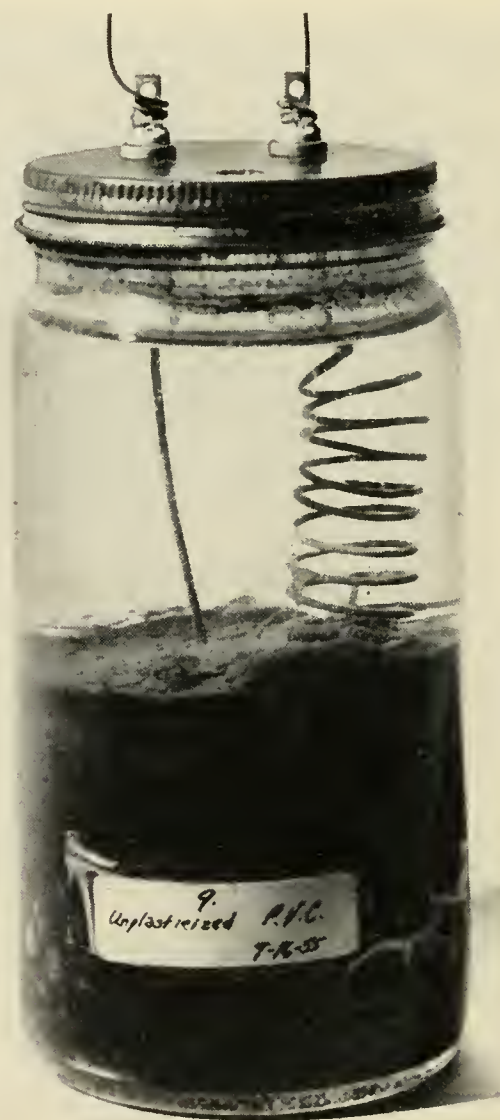
Fig. 5 - General setup of conductor test showing a coil half in sediment and half in sea water.
