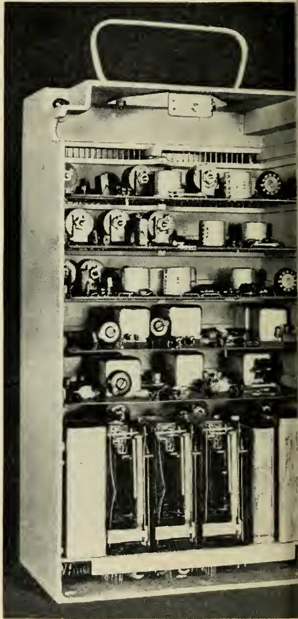
Fig. 18 — Typical terminal network mounted in a prototype connector box.
