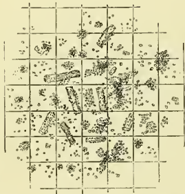
Microscopic Appearance of Common Calcined Magnesia.
