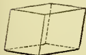
Oblique rhombic prism (principal form of sulphur by fusion and slow cooling).
