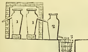
Distillation of Native Sulphur.
