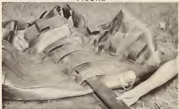
Starting with the bottom stave pocket, stave is inserted through its five pockets.
