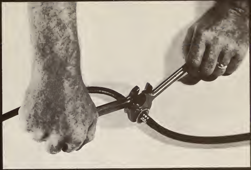
D. Attach end of hose taken from yoke assembly to end of hose extending from Oxygen cylinder. Use two wrenches (m) as shown to tighten securely.
