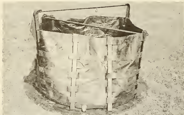
Tank is raised and supports matched with stave caps, using straight and cotter pins.
