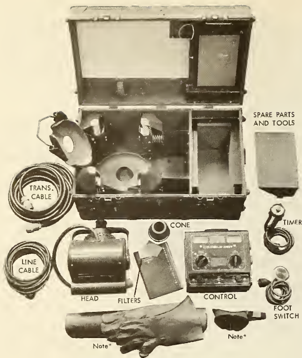
TRANSFORMER, TUBEHEAD AND CONTROL CHEST
