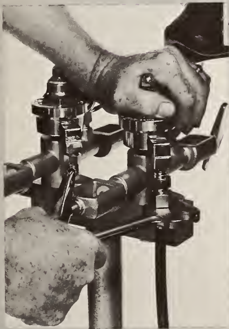
D. Disconnect hose from Nitrous Oxide side of yoke assembly.
