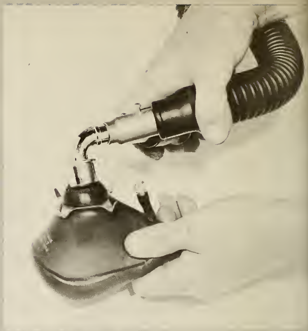
B. Fit large end of adapter (j) into opening in mask (c).
