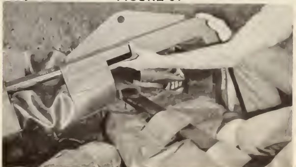
A long aluminum cap is slipped over the top of a stave and pocket assembly, per instructions. FIGURE 62
