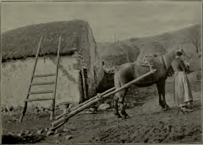
FIG. 2. Slide-Car, County Antrim ; from a photograph by the Author.
