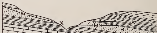
FIGURE 9.—Diagram illustrating manner of formation of spring at contact of pervious formation and impervious formation when dissected. A, C, Impervious shale beds; B, porous water-bearing sandstone; M, top of saturated zone; X, point of emergence of spring.
