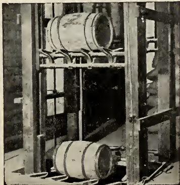
Elevator for barrels, casks, etc. Capacity, 600 per hour.
