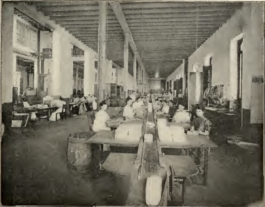
Hand Packing Department at the "El Siboney" factory, Havana. Cigarettes seen in the belt conveyor are of the well known brand of Cabañas. The cigarettes are packed by women and tied in bunches of 26 packs. The room is well ventilated and kept clean. The belt conveyor takes the bundles down to the floor below, where they are packed into boxes for export or sent out in boxes for the city delivery.
