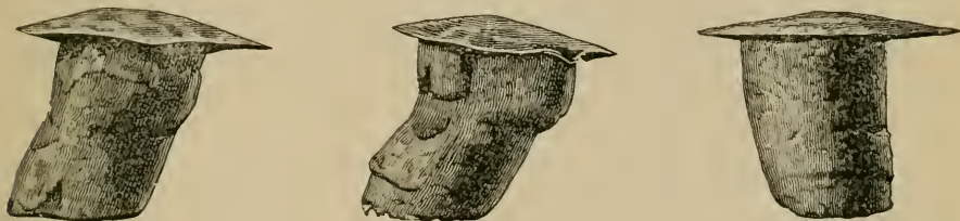
SOME DEFECTIVE RIVETS.
