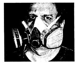
The 3M 601 Adapter positioned for sampling behind the cartridge. The tubing is pinched closed until the air sample is taken.
