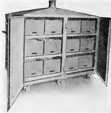
Fig. 153.—Combined sterilizing oven and truck. (A. H. Barber Creamery Supply Co.)
