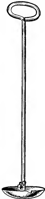
Fig. 28.—Combined cream stirrer and sampler (Van Slyke).
