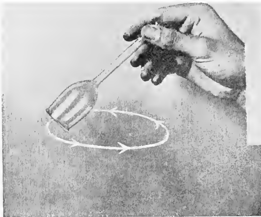
Fig. 43.—To mix the acid and milk shake the bottle until the contents are of a uniform brown color. (Circular of Information No. 27, July, 1916, Univ. of Wis. Agri. Exp. Sta.)
