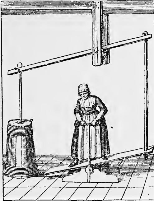
Fig. 4.—Churn operated by foot power (Benno Martiny).
