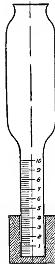
Fig. 66.—Casein tube and eork support. (Bull. 156, November, 1907, Univ. of Wis. Agri. Exp. Sta.)
