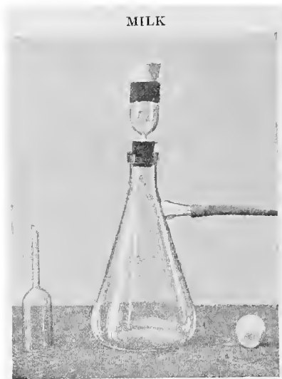
Fig. 80.—Gooch filtering apparatus, showing also unassembled parts, e. g. , porcelain Gooch crucible, with perforated sieve bottom, glass Gooch funnel, and pressure tubing leading to Chapman pump. (Tonney, Amer. Jour. of Public Health, 1912, vol. 2, p. 280.)
