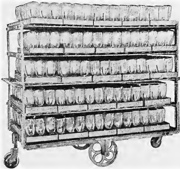
Fig. 156.—Special steel frame bottle truck.
