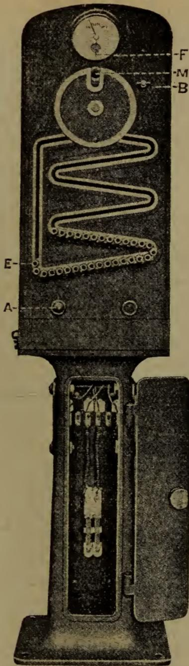
**FIG. 120.** ABSOLUTE STAFF INSTRUMENT WITH PEDESTAL.
