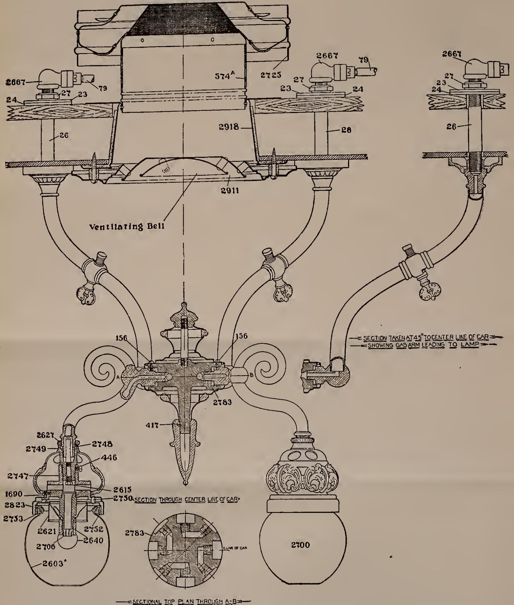
FIG. 55. SECTIONAL VIEW OF LAMP—DETAILS AND PARTS SHOWN.
