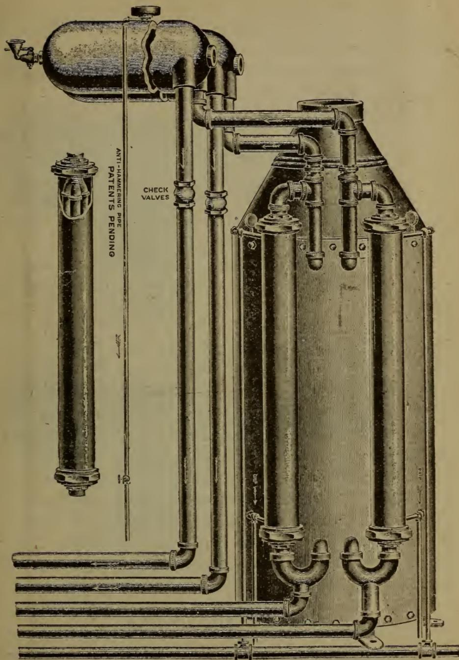
FIG. 9. DETAILS OF IMPROVED BAKER STEAM ATTACHMENT.
