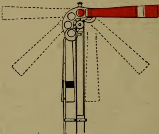
FIG. 105. DIFFERENT TYPE OF THREE-POSITION SIGNAL. "STOP"-HORIZONTAL; "CAUTION"-INCLINED; "PROCEED"-DOWN.
