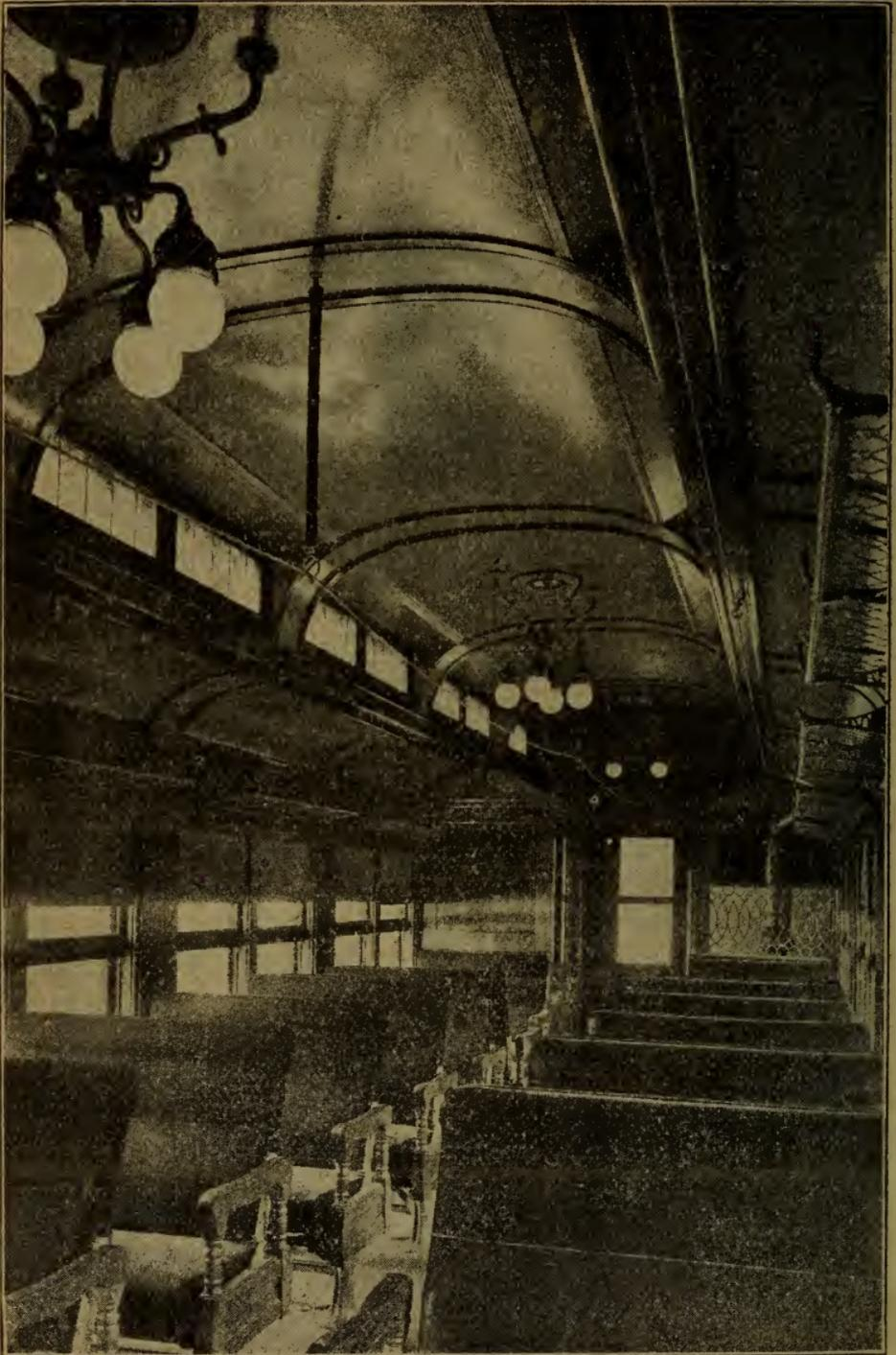
FIG. 57. INVERTED BURNER LAMPS IN PASSENGER COACH.
