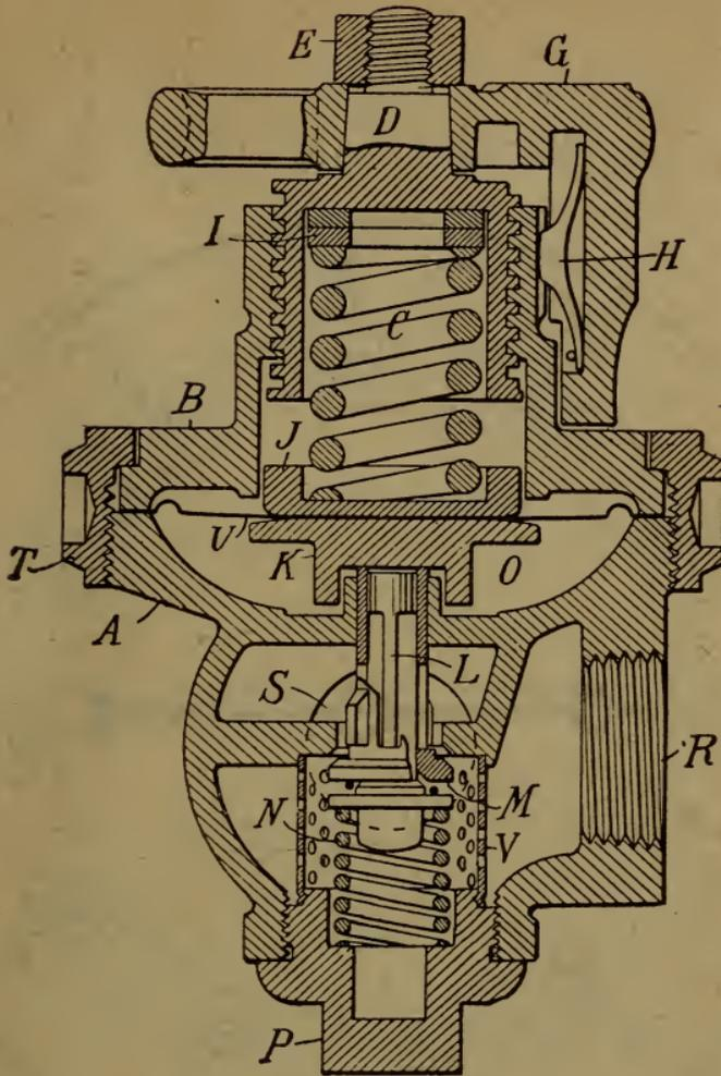
FIG. 27. SECTIONAL VIEW IMPROVED TEMPERATURE REGULATOR.
