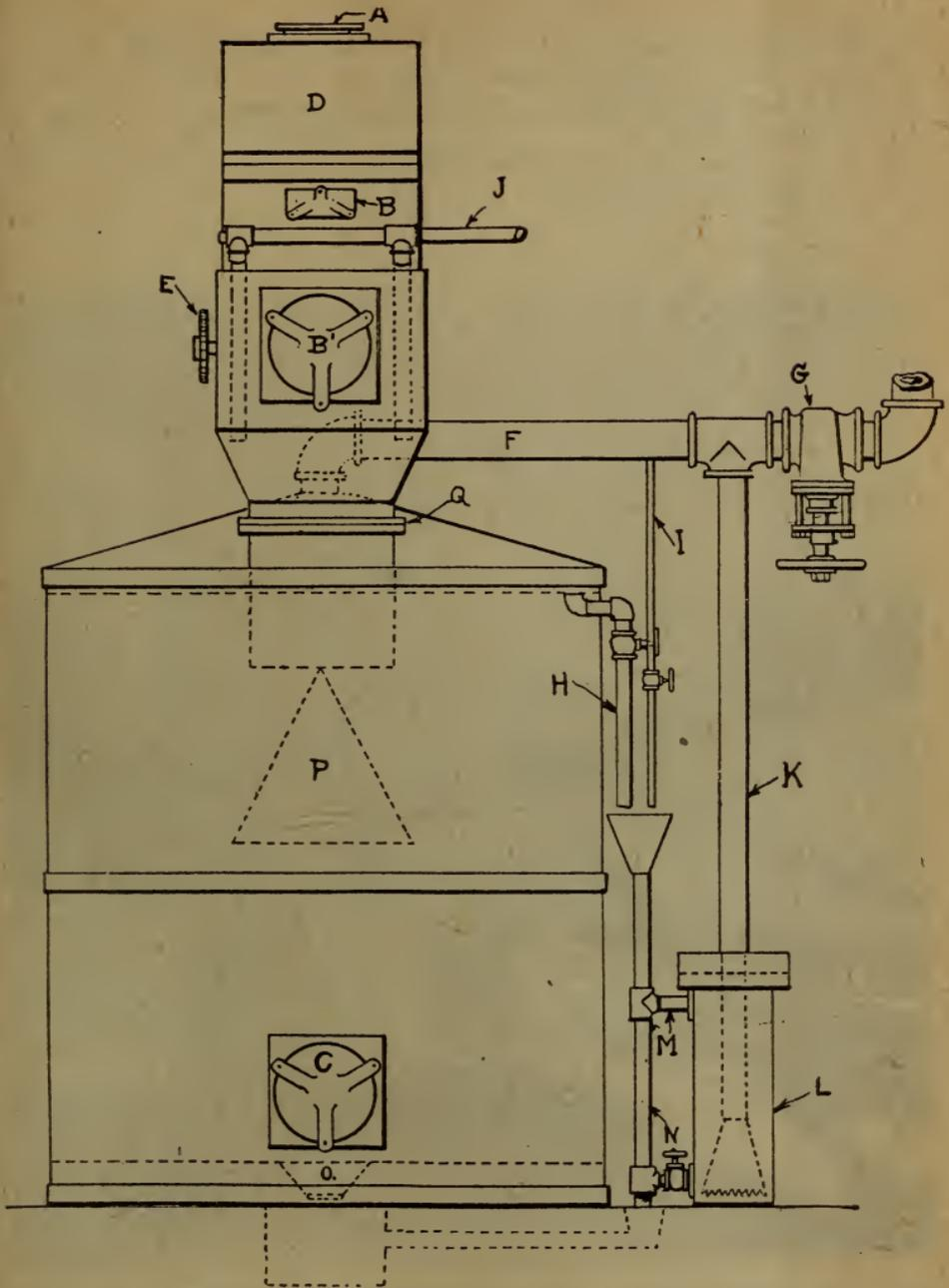
FIG. 66. GENERAL ACETYLENE GENERATOR.
