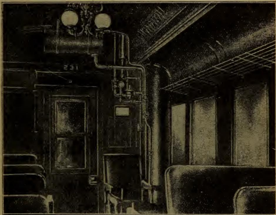
FIG. 59. INTERIOR OF COACH, WITH GAS GENERATOR INSTALLED.
