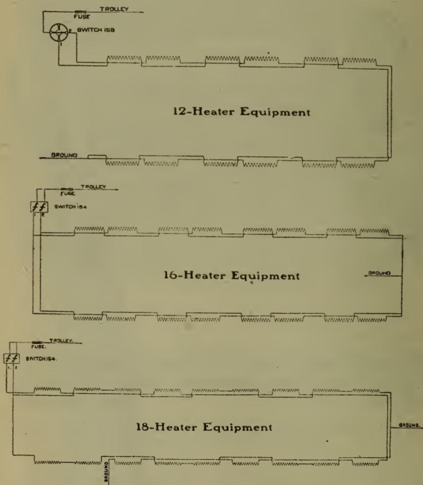
FIG. 42. DIAGRAMS OF WIRING ELECTRIC HEATING SYSTEM.
