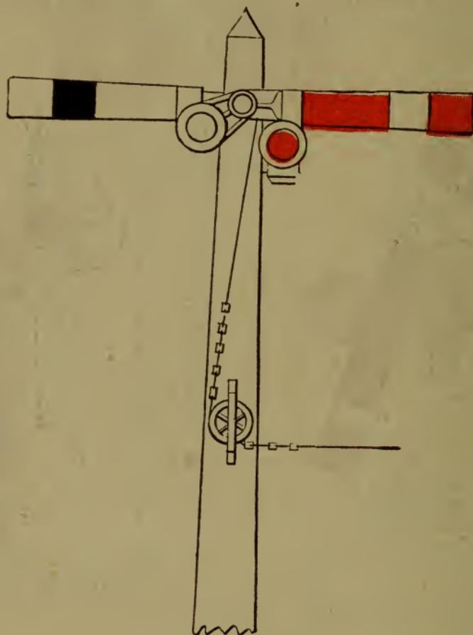
FIG. 102. A TWO-POSITION TRAIN-ORDER SIGNAL.
