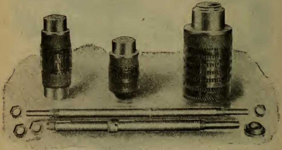
FIG. 84. ARMATURE SHAFTS AND NUTS OF GENERATOR AND BUCKER, SHOWING SPIDER AND REMOVABLE SHAFT CONSTRUCTION.
