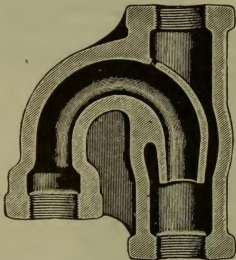
FIG. 32B. SECTIONAL VIEW DUPLEX COILS.
