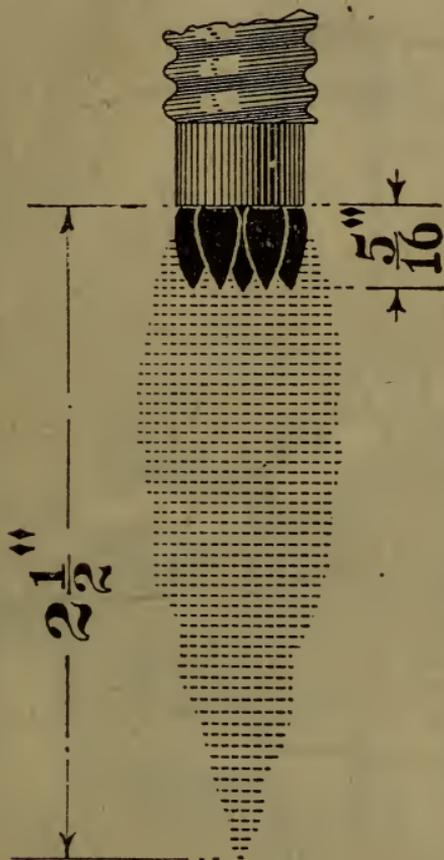
FIG. 56. SHOWING PROPER FLAME.
