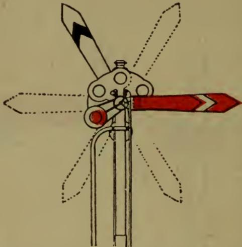
FIG. 104. A THREE-POSITION SIGNAL. "STOP"-HORIZONTAL; "CAUTION"-UP; "PROCEED"-DOWN.
