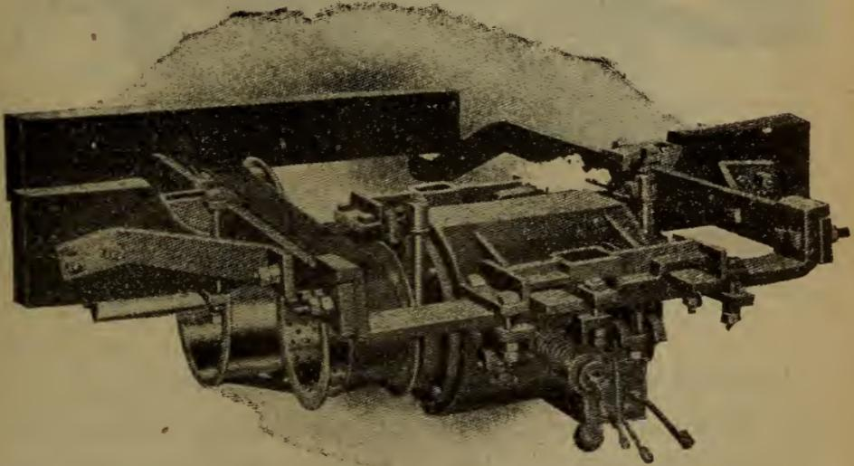
FIG. 78. CAR GENERATOR SHOWING OUTSIDE SUSPENSION, PULLEY END.
