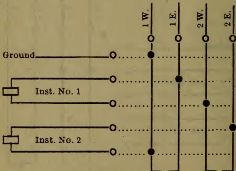
Inst. No. 1 on No. 1 E. to No. 2 W., Ground on No. 1 W.
