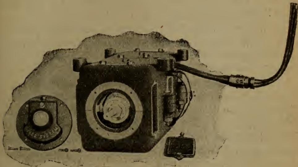
FIG. 92. END VIEW OF BUCKER SHOWING COMPLETE COUPLER HEAD AND BLOCK AND METHOD OF CONNECTING CAR WIRES. BEARING HEAD AND HAND HOLE COVER REMOVED EXPOSING MOTOR COMMUTATOR.
