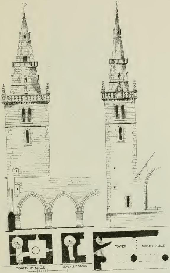
FIG. 1270.—Cupar-Fife Church. Plans and Elevations of Tower.
