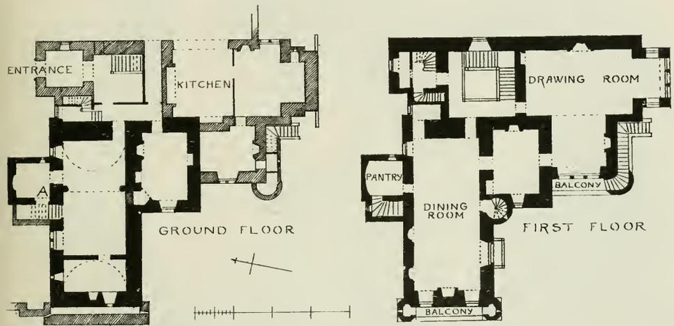
FIG. 1401.—Grange House. Plans of Ground Floor and First Floor.
