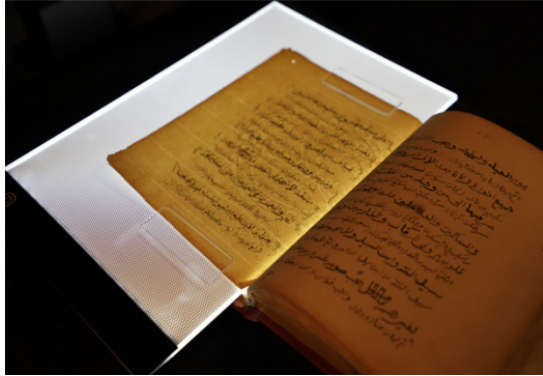
Paper position on LED lighting board for watermark shooting. Photo by Abdullah Maulani CC BY 4.0.
