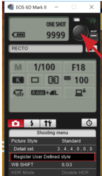
Shutter remote camera button on Canon Remote Shooting app. Captured by Abdullah Maulani CC BY 4.0.
