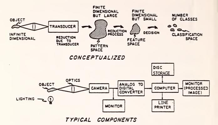
Fig. 1. Typical electronic recognition system.
