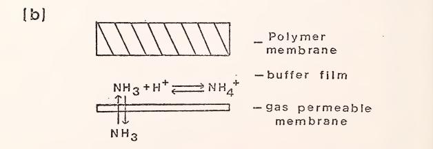
Figure 3 a) Schematic diagram of new ammonia sensor.
