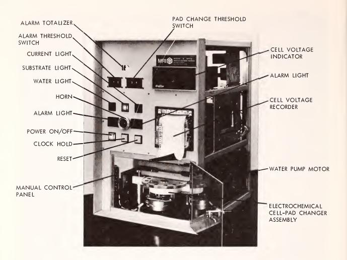
Figure 3 - Continuous Aqueous Monitor (CAM-1)
