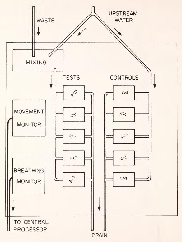
2. An inplant monitoring system with control fish exposed to dilution water only and test fish exposed to a mixture of wastewater and dilution water.
