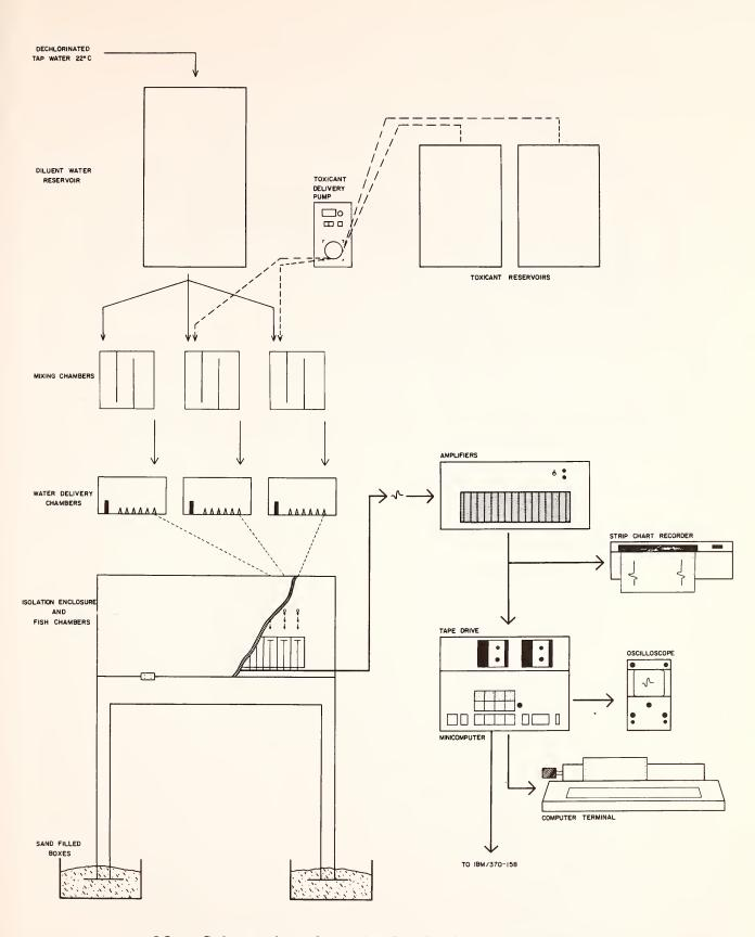
13. Schematic of variable dosing apparatus.
