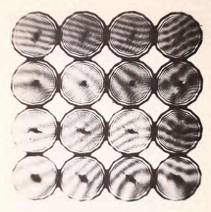
6. Twelve optical spatial filters positioned on a 2" X 2" glass plate. Since the size of each filter is generally inversely related to the size of the input image, approximately 100 such filters can be placed on a single plate.
