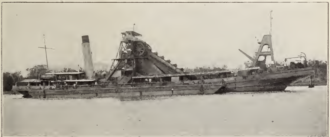
The Corozal, the newest and most modern ladder dredge in the Canal service. It is equipped with five yard buckets and can dig to 45 feet below mean sea level.
