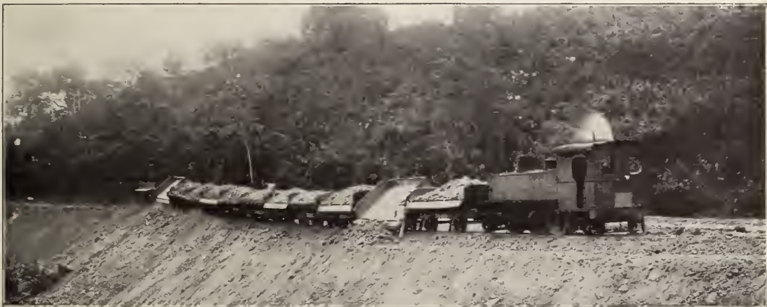
Old French dump cars. Steel cars, 18 feet long, were used exclusively. The cars dumped on one side only, and were too small for economical use. Most of these were scrapped by the Americans.
