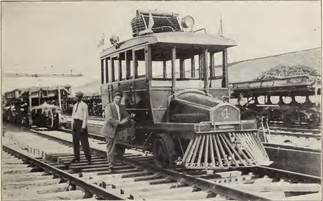
Colonel Goethal's motor car, commonly known as the "Yellow Peril" from its color; also as the "Brain Wagon." Several of these cars have been shipped to the Isthmus, and are used by the officials in inspecting the different parts of the work.
