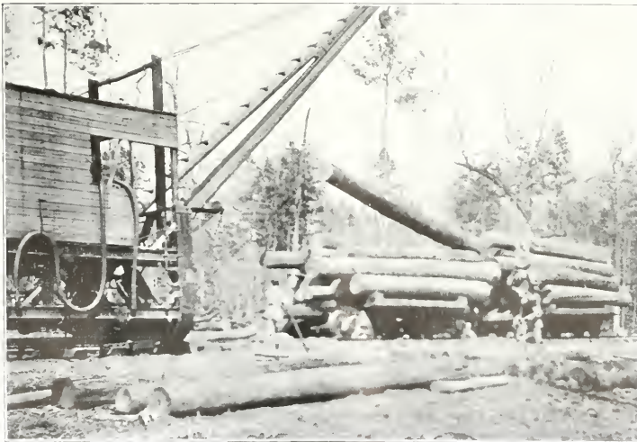
GETTING LOGS ON THE CARS WITH A LOG LOADER
