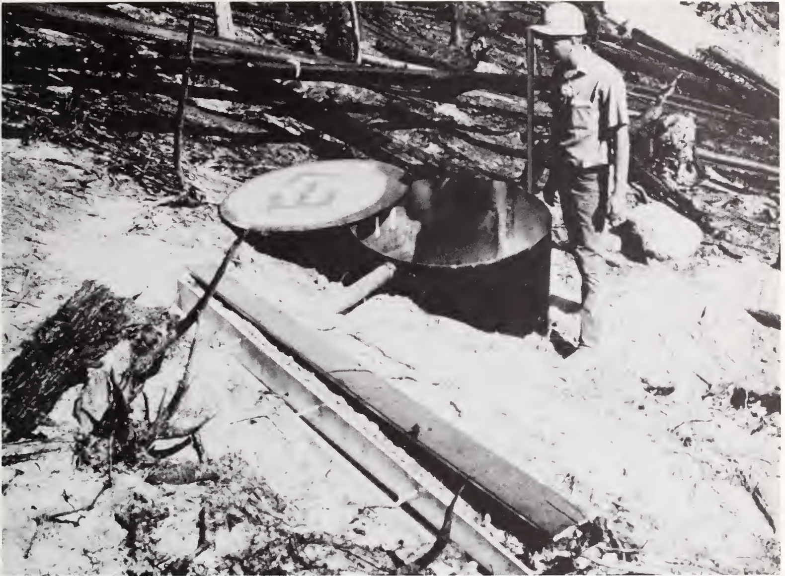
Catchment trough and storage tank installed immediately after burning at the base of a runoff plot at Miller.
