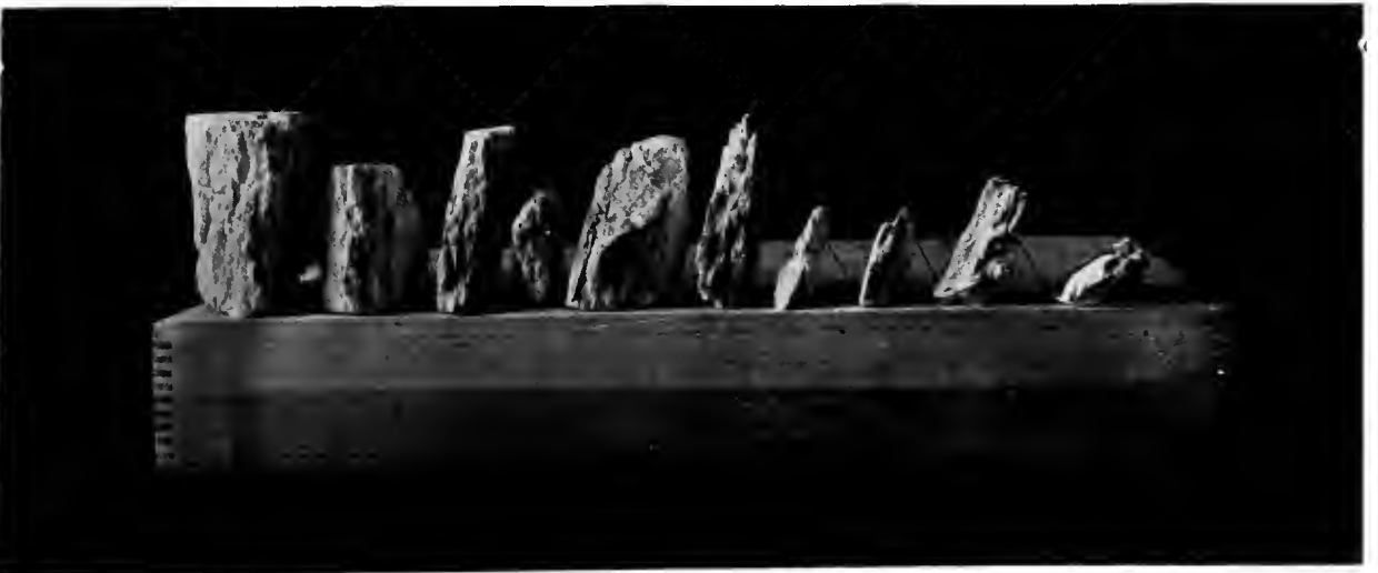
PIECES OF VARIETY "A" SO PLACED AS TO SHOW THE SLATY STRUCTURE NOT ONLY AT RIGHT ANGLES TO THE BEDDING PLANES BUT ALSO AT OTHER ANGLES WHEN COMPARED WITH THEM. THE BOTTOM OF EACH SPECIMEN REPRESENTS AN ORIGINAL BEDDING PLANE. (GREATLY REDUCED.)
