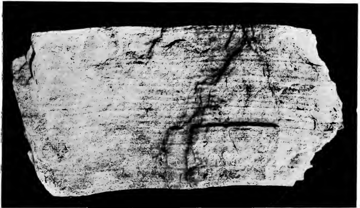
PIECE OF VARIETY "A" OF THE METAMORPHOSED WHITE OR GRAY SANDSTONE SHOWING ORIGINAL BEDDING PLANES.
