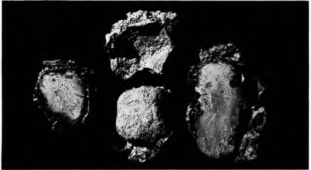
TYPICAL SHALE BALLS WITH NICKEL-IRON CENTERS. Note the Widmanstätten figures shown on the two specimens which have been sawed in two. Greatly reduced.
