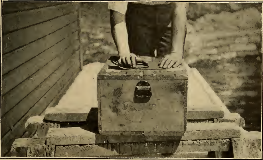
FIG 3. USING EMERY CLOTH TO SMOOTH DOWN A RING THAT BINDS IN ITS GROOVE
